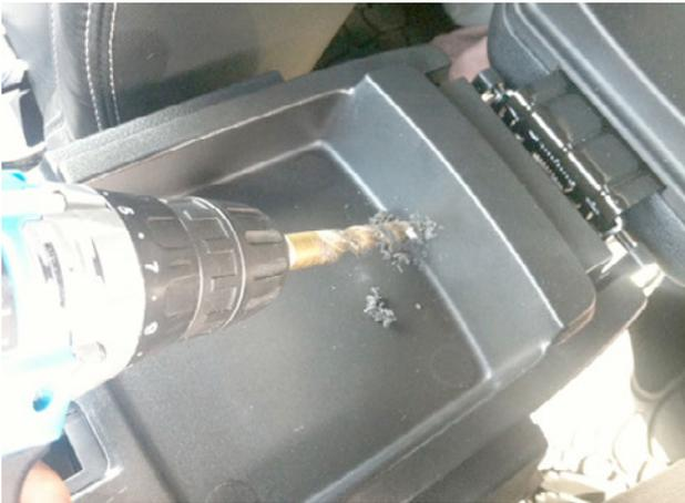
**Step 3:** Route plug of Charging Module through 1/2" hole and place module in tray.
