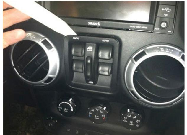
**Step 11:** Disconnect harness from window switches.
