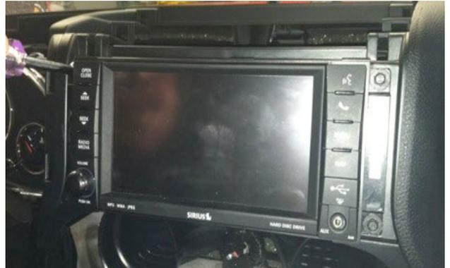
**Step 16:** Using a plastic trim removal tool, remove HVAC panel to access power point.
