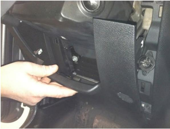
**Step 14:** Remove (2) 7mm bolts on both sides of the steering column.
