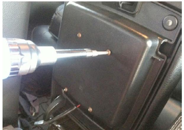
**Step 5:** Using Trim Removal Tool remove hinge cover.
