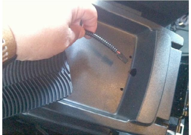
**Step 4:** Align the (4) 3/16" holes with mounting holes on module and insert the (4) 3/8" Pan Head T-15 Torx Screws through tray into module.
