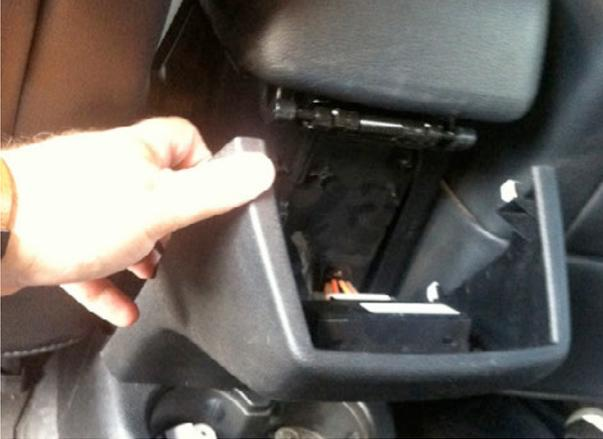
**Step 7:** Drill 1/2" hole through lower armrest bin side panel 1 1/2" below top lip on passenger side of vehicle.
