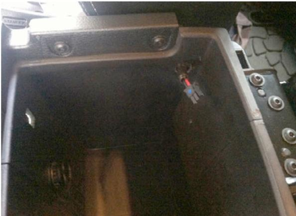
**Step 20:** Connect Power Harness to Charging Module.
