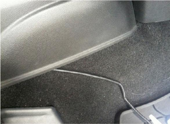
**Step 19:** Run harness through 1/2" hole into armrest bin.
