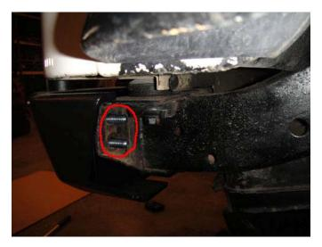
**11.** Next install the last 4 bolts using the mounting plates from step 7. Place the mounting plates up behind the cross-member.
