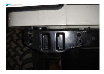
2. This applies to TJ's and YJ's Only. Note: Unlimited's do not need to do this step. Remove the 4 nuts across the rear cross-member that attaches the gas tank skid plate to the frame.
