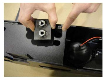
8. With the help from a friend, place the bumper up to the rear and bolt the bumper up in place using the 2 factory bolts removed from the bottom of the frame. Leave these bolts loose so you can install the rest of the bolts and have a little movement of the bumper. They will be tightened at the end. These will hold the bumper up in place while you install all of the other bolts.
