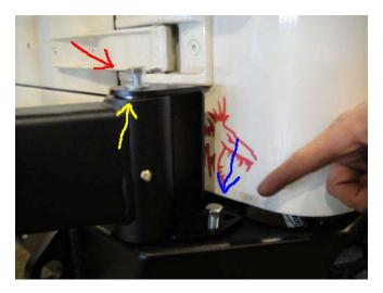
**19.** Install the latch using the supplied  $\frac{1}{4}$ " x  $\frac{3}{4}$ " fine thread bolts. Apply Locktite to these bolts and do not overtighten them.
