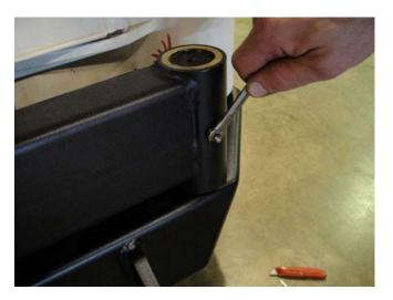
**18.** Next install the pin brace using 4 (3/8" x 1") bolts. Three of them will bolt into the bumper as shown by the blue arrow and 1 will thread into the Spindle as shown by the red arrow. NOTE: install a washer on top of the spindle between the spindle and pin brace as shown by the YELLOW arrow. This prevents the brace from contacting the carrier when it is rotated open and closed.
