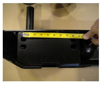
the vertical scribe marks. Now measurement the distance between the two vertical scribe marks on the rear cross-member and compare that to the two inside sets of holes on the bumper. This measurement will confirm proper fitment of holes.
