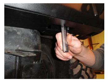
**13.** Next apply grease to the hinge pin. Smear a small amount all over the pin before installing the tire carrier.
