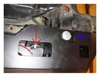
**12.** Align/Center the bumper side to side with the body. Also be sure the bumper is level across the back. Once the alignment is correct tighten all of the mounting bolts.
