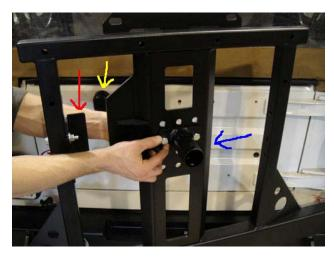
**NOTE**: We supply 2 of these L-Brackets and the other one is used on the passenger side (not shown) and makes contact with the rubber isolator on the passenger side. Its recommended that you install both of them to prevent any rattling.
