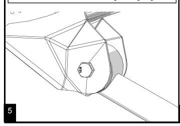
Install the flex-joint side into the axle bracket with the cam bolt. Rotate the cam bolt until it has shifted all the way forward. Tighten finger tight. Repeat steps 2-6 for the remaining front lower arm, then lower the vehicle and torque the cam bolts to 85 ft-lbs and frame side bolts to 130 ft-lbs.
