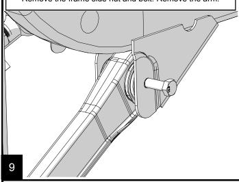
Slide the bushing side of the flex arm into the frame side
