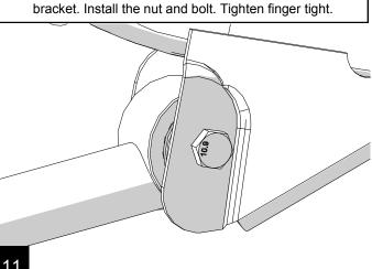
Install the flex-joint side of the arm into the axle side bracket. Tighten finger tight. Repeat steps 8-12 for the remaining rear lower arm. Lower the vehicle and torque all bolts to 130 ft-
