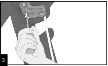
**Note:** The Axis Sun Visor has 2 friction setting bolts and 4 mounting bolts. The upper 4 mounting bolts (pictured) should be kept tight and not be loosened to adjust rotational stiffness. The lower two bolts can be tightened or loosened to adjusted for rotational stiffness.
