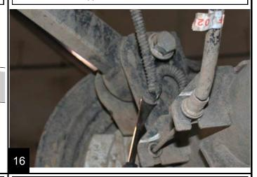
Remove the parking brake cable bracket from the underside of the body with a 10mm deep socket and discard.
