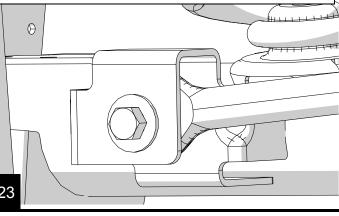
To straighten the steering wheel, loosen the adjuster sleeve on the drag link with a 15mm. Make a mark across the sleeve and threads to indicate the original position. Looking from the drivers side, rotate the adjuster sleeve counter clockwise 3/4 of a turn. This should be pretty close. Every vehicle is different, test drive yours and adjust as needed. Torque the pinch clamp bolts to 45 ft-lbs.
