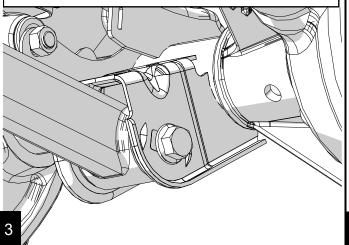
Remove the shocks at the axle with an 18mm wrench and socket. (See 999207 Shocks/Front/Removal)
