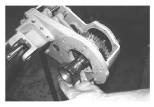
3. Install the thrust washer.
