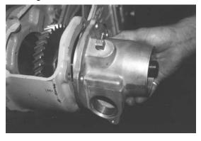
9. Install the end play shims on the rear output shaft.
