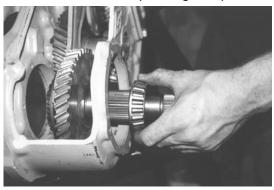
6. Insert the speedo gear and then the outer speedo
