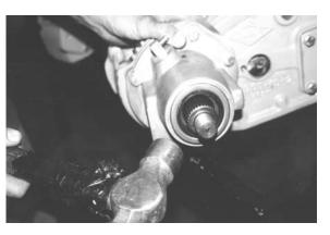
14. Install the rear output shaft yoke and tighten the locknut to 90-100 ft. lbs.
