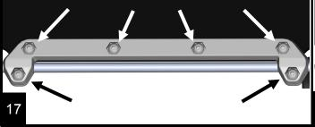
Use a 3/16" drill bit to drill a hole through the roll bar using the hole in the visor mount as a pilot hole (one per mount). Note: Place a blanket or plastic over the seats and carpet to avoid getting metal shavings on them. Install the rivet through the mount and into the hole just drilled out in the roll bar. Use pop rivet tool to attach the
