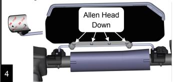
Install the rivet through the mount and into the hole just drilled out in the roll bar. Use pop rivet tool to attach the rivets.
