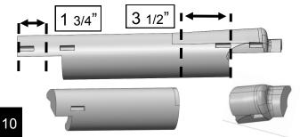
**Note:** Allen bolt heads must be facing downward, when the visor is in the up position, for adjustment. Next, remove adhesive backing form visor mounts and, using the marks made on the roll bar as a guide, attach the Axis Sun Visor.
