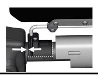
For a soft top the visor mounts need to be turned in (see image below). The head of the allen bolts in the mount needs to be facing downward for ease of visor removal. With a 1/8" allen, remove the bolts and flip them around (tighten enough so the hardware doesn't fall out during install).
