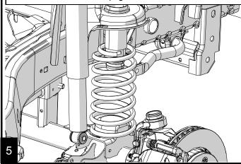
Locate the center of the spring pad and drill a 5/16" hole for standard pad installation. For speedbump pads, drill a 3/8" hole.
