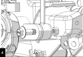
Lower the axle and remove the springs. (See Springs/Front Removal 999206) Upper bumpstop extensions installation see page 5 now.
