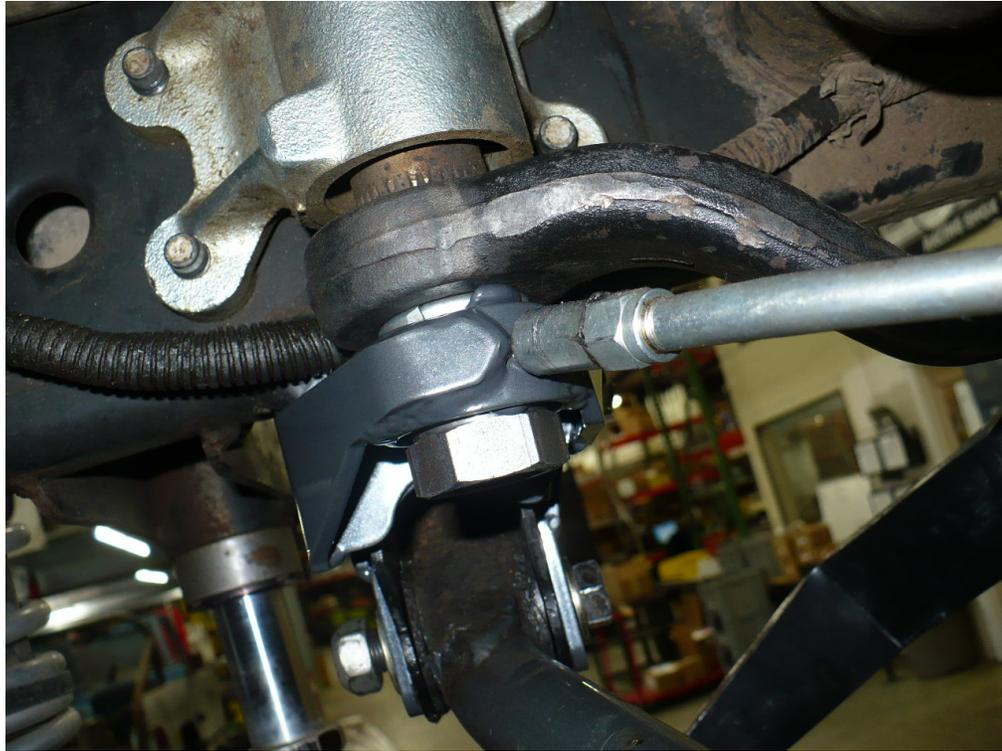
20) Recheck all hardware after 100mi of driving and during normal post / pre off-road bolt checks.
