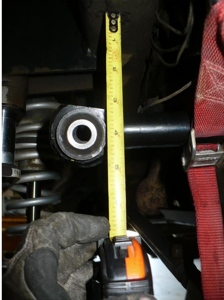
Bump stop measurement shown from bottom of frame to mounting hole with stock Track Bar.
