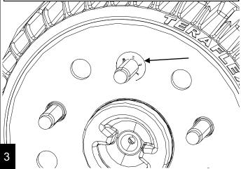
Slide the adapter onto the wheel studs and use a straight edge to verify that the studs do not protrude.
