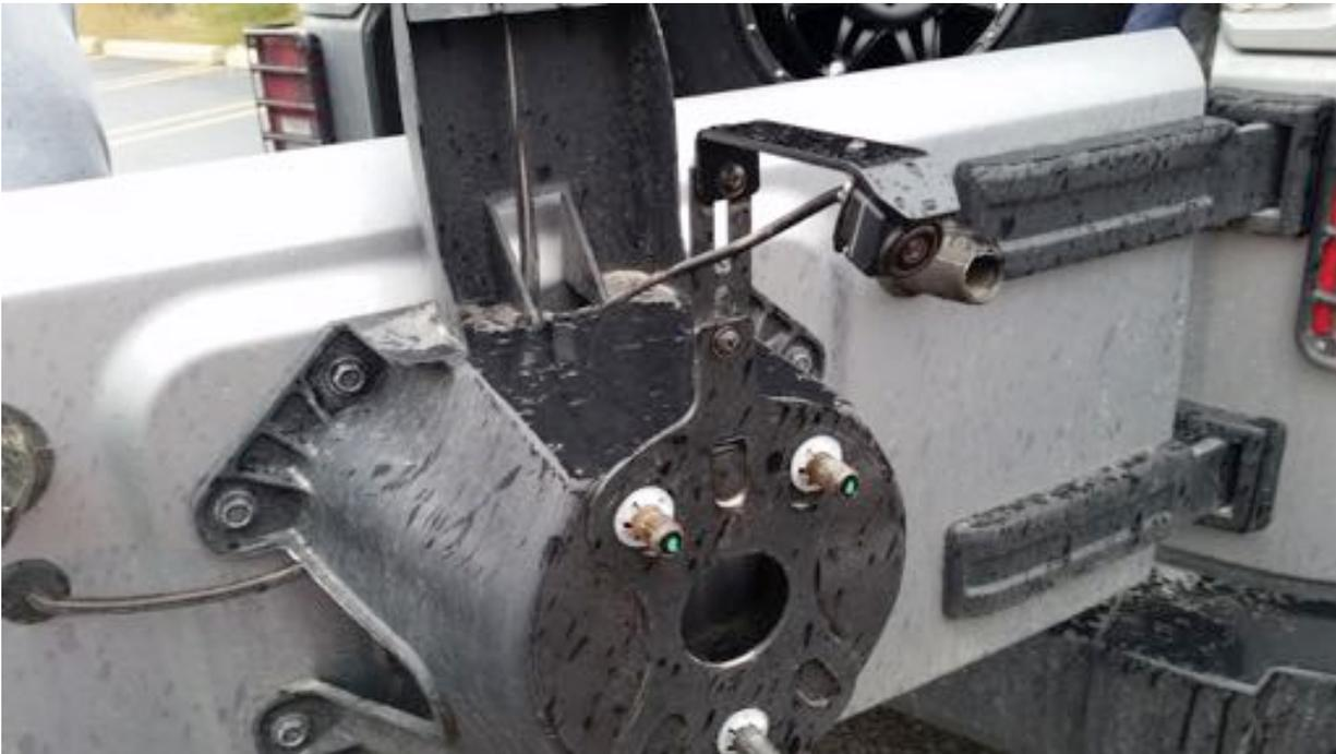
Adjustment Bracket for Camera Clearance using Phillips Screwdriver and 3/8" Wrench or Socket Drive
