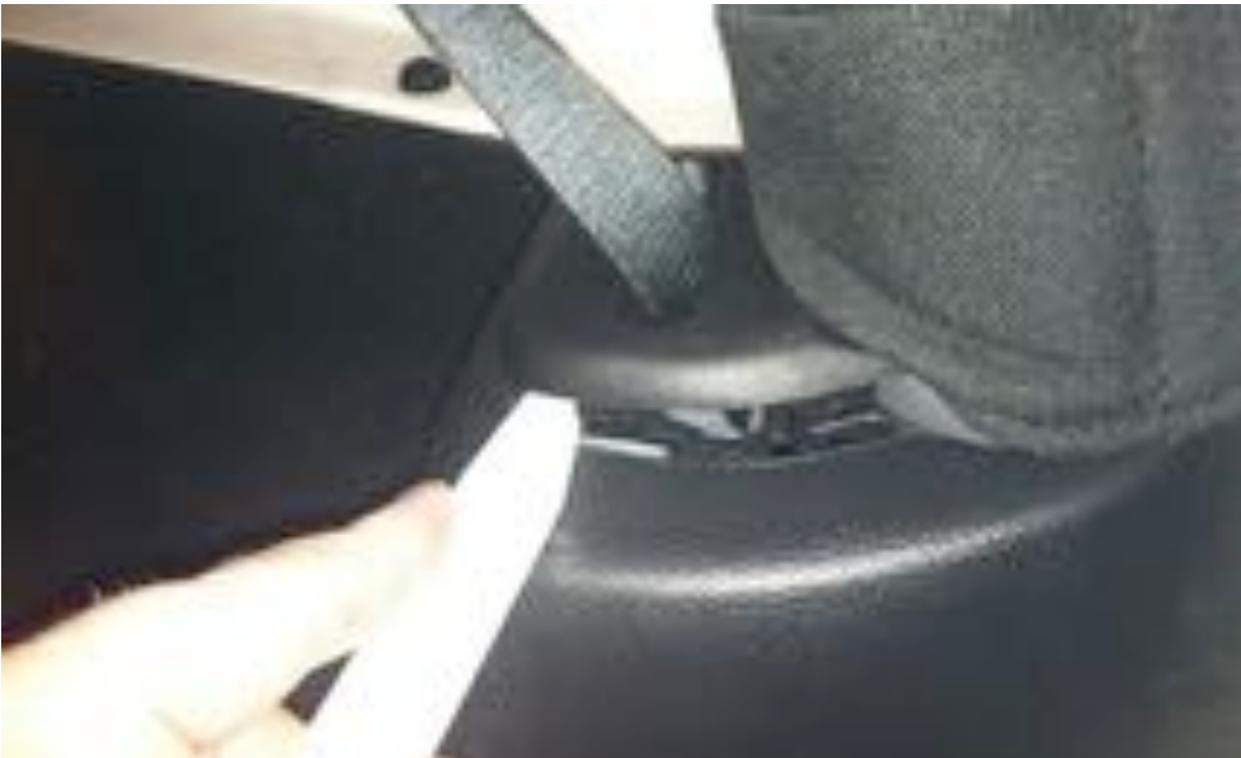
9. Using a plastic trim removal tool, remove rear access panel to expose 10mm bolt, and remove bolt.
