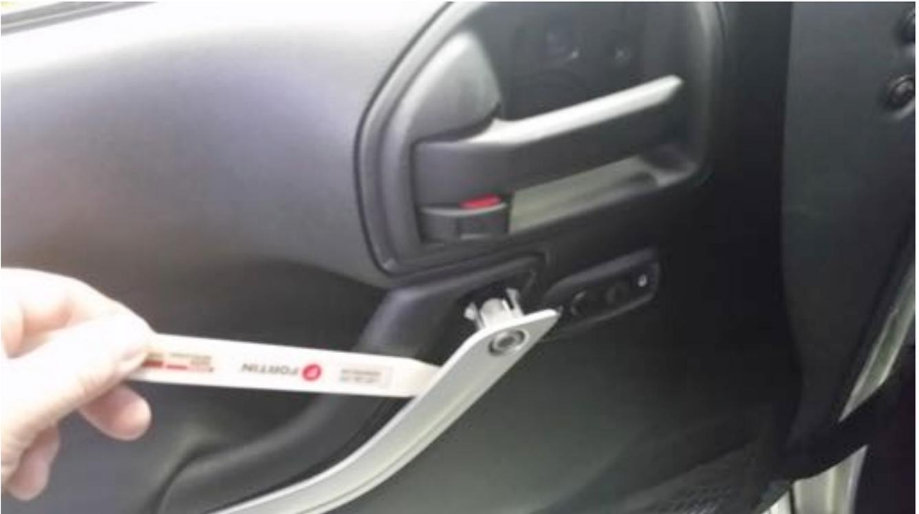
5. Remove the (2) Torx in the lower front of the door.
