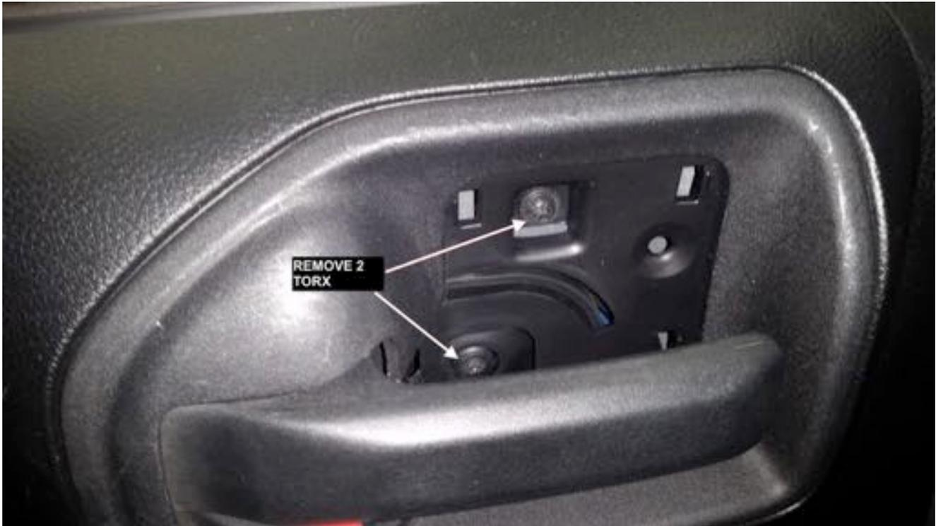
4. Remove the inter trim on the pull handle to gain access to the two screws behind the trim.
