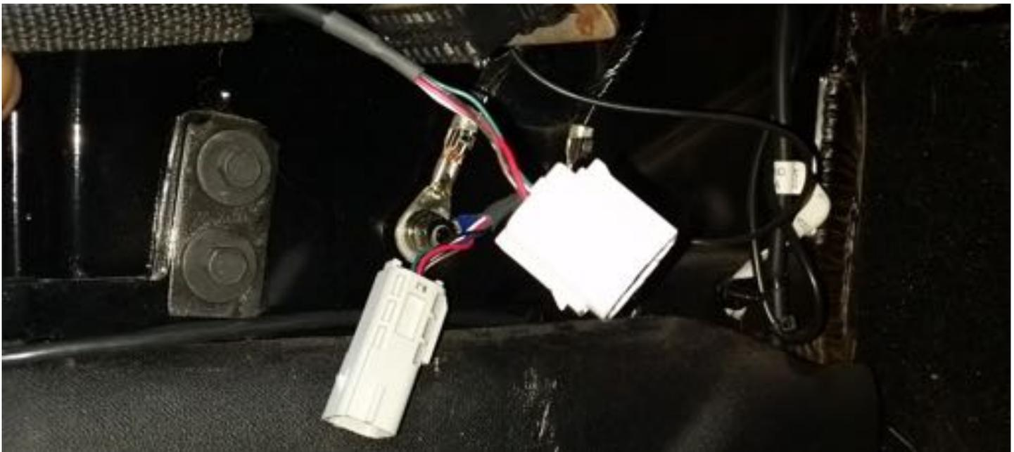
26. Run the camera wire to behind glove box area to connect to the 360° main control module. (Passenger side camera harness may have excess length, coil excess and zip tie behind passenger kick panel.)
