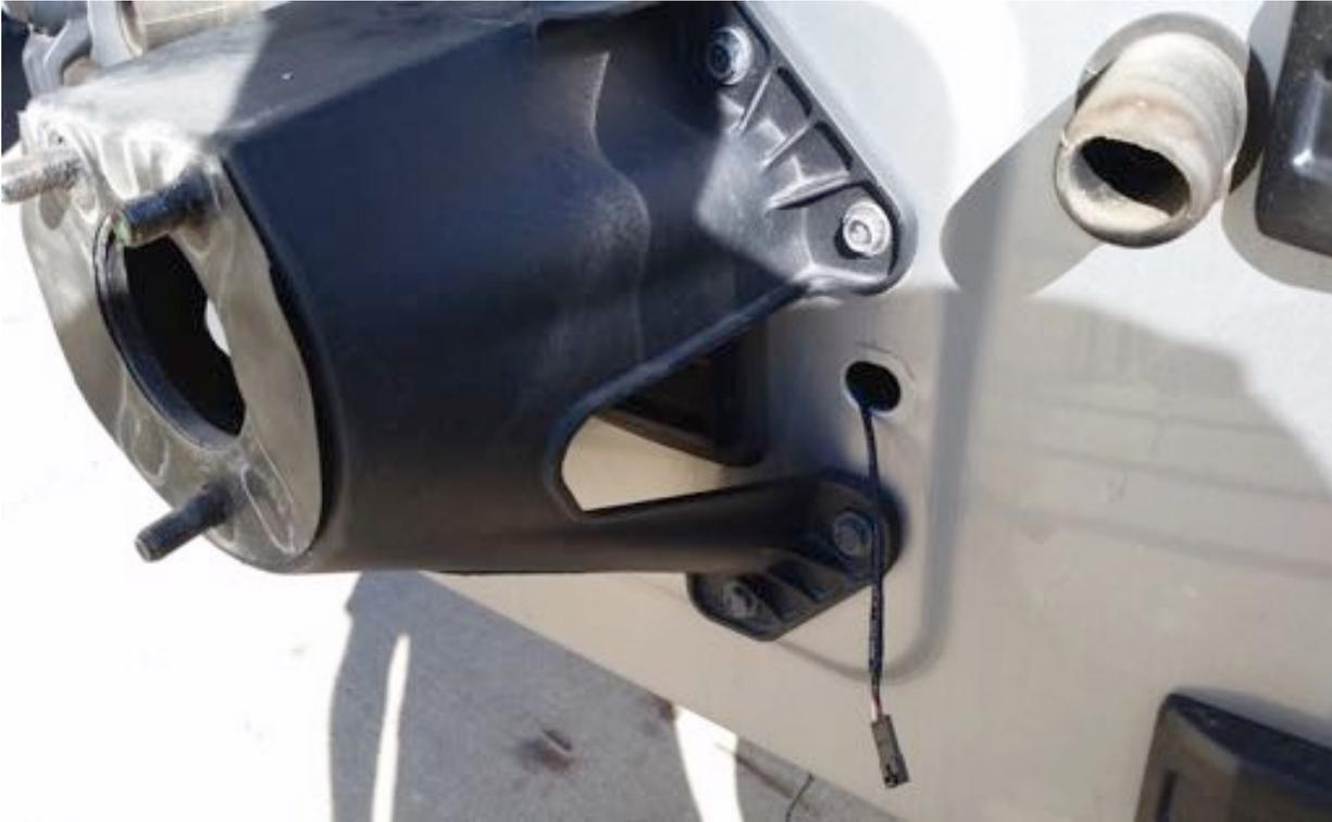
5. Run rear camera harness through top hole of tire carrier.
