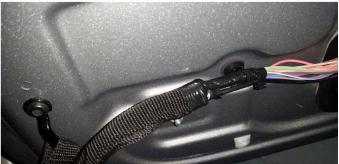
25. Secure the harness in the kick panel so that the door removal connector is located in the same location as the factory door connector.
