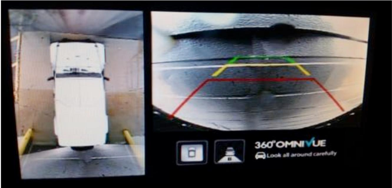
11. Shift back into park. Press the power button on the 2 button keypad once to see if the 360° image comes up on the screen. To shut off the system press the power button 3 times in 1 second.
