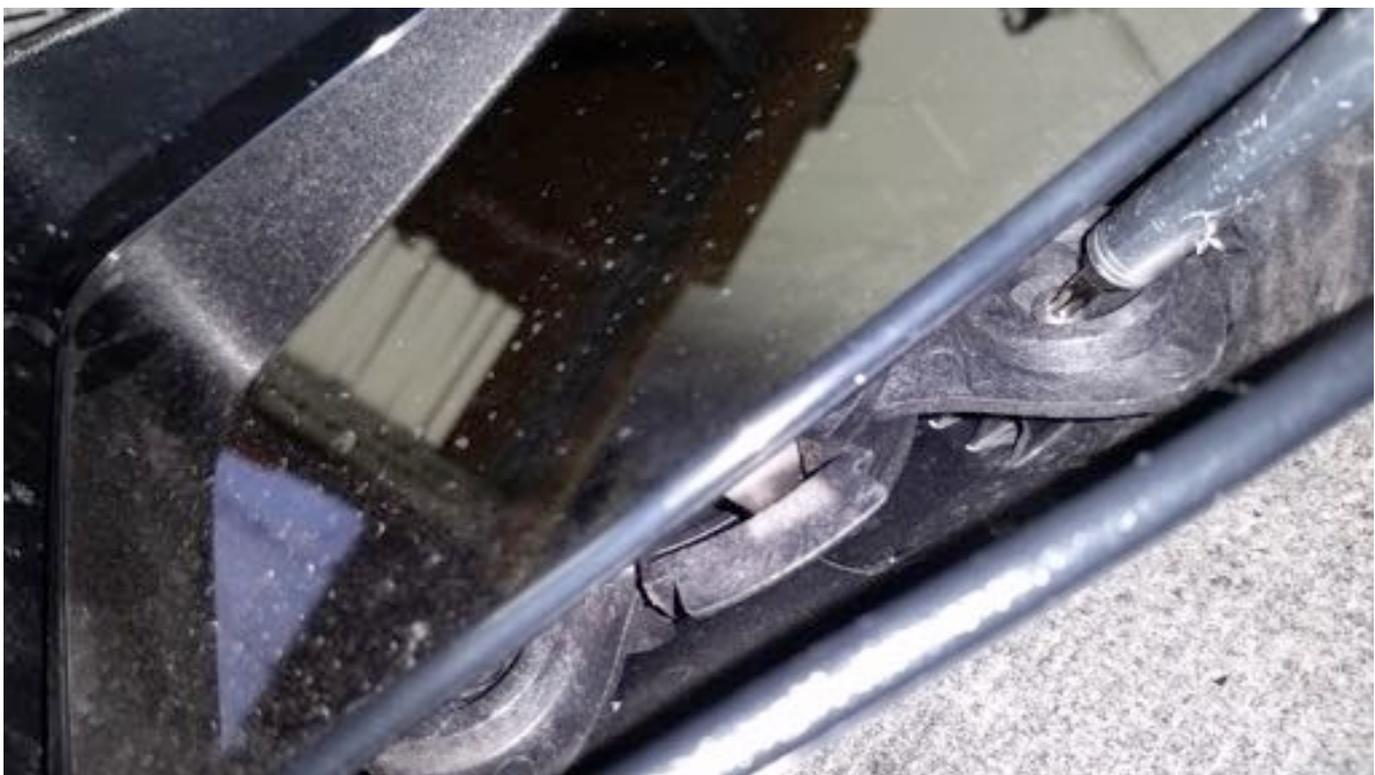
12. Remove the mirror glass by gently lifting on the plastic tabs holding the glass to the mirror motor.
