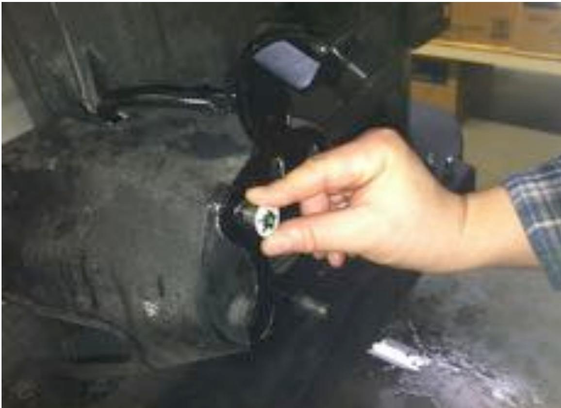
4. Run the harness into the rear gate through the factory grommet.
