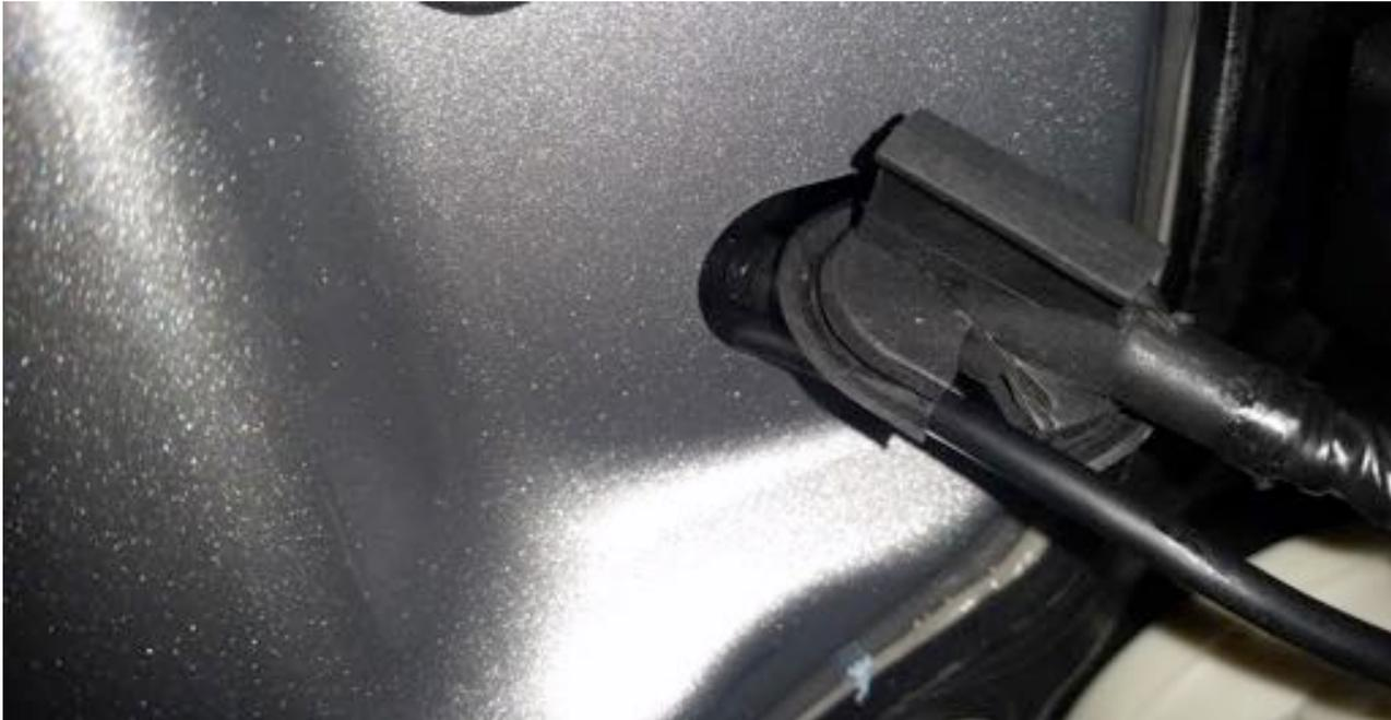
19. Notch the grommet to allow room for the camera harness.
