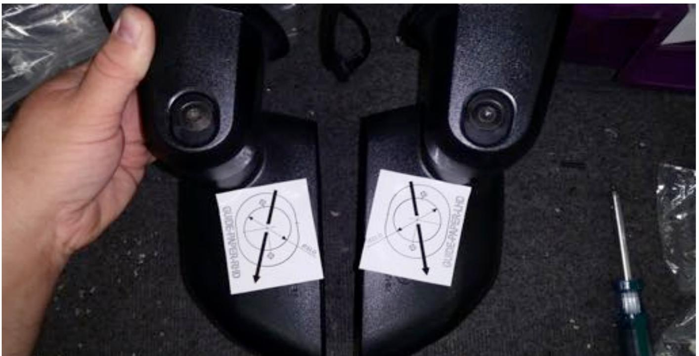
11. Remove the (3) Torx screws from inside the mirror. You can fairly easy get behind the mirror glass to do this. (The picture show the glass already removed to show location of the screws).
