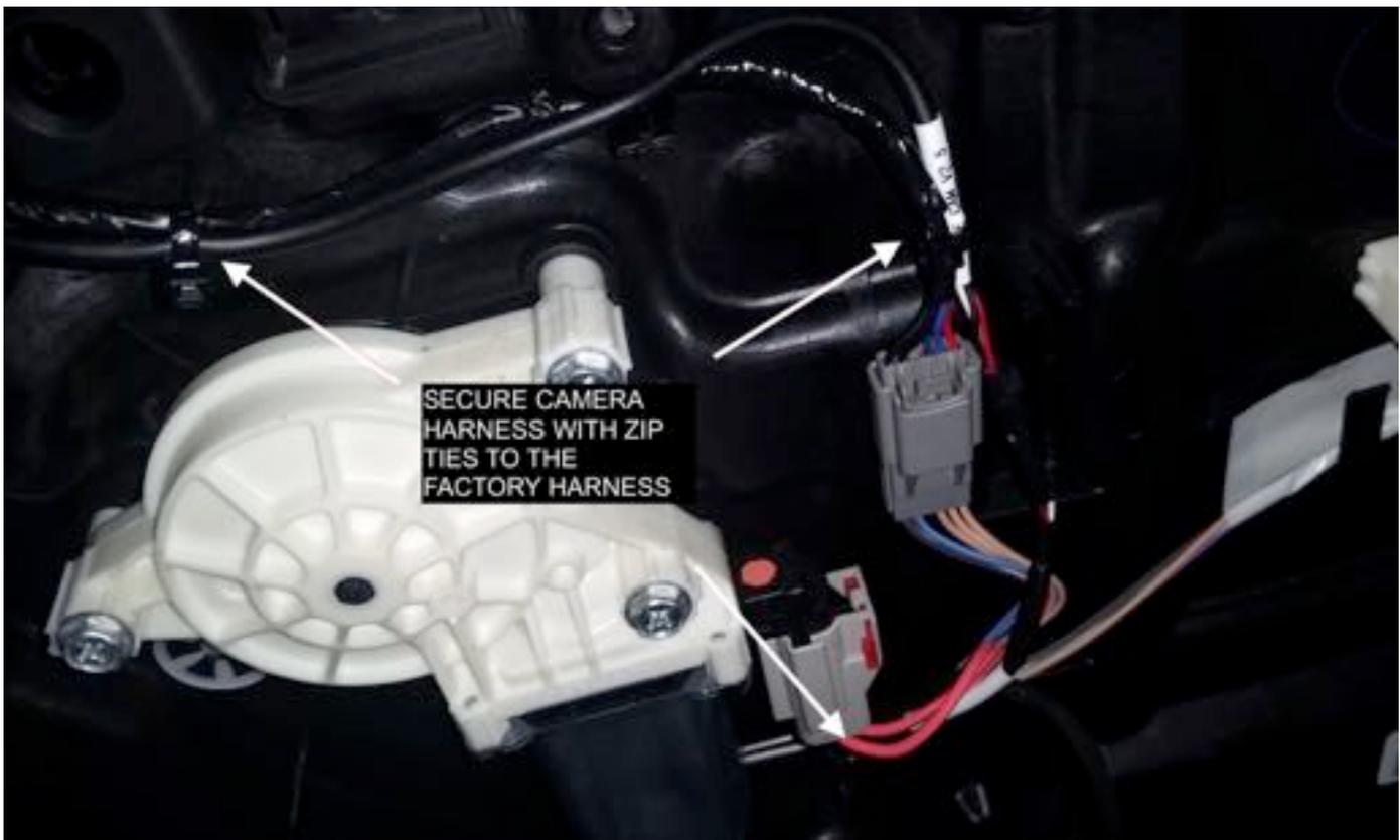
24. Run the camera wire through the factory door sleeve. Use a long zip tie or a fish tape.
