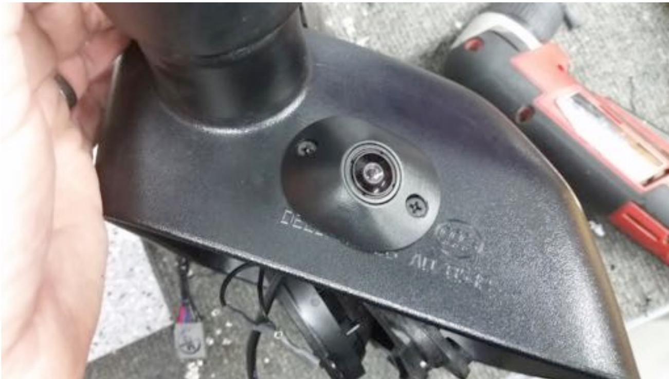
16. Tape the terminals to a zip tie to help guide the wire through the back of the mirror and mounting arm. Run the camera harness through the back of the mirror where the factory power harness passes through and out the bottom of the mirror arm.
