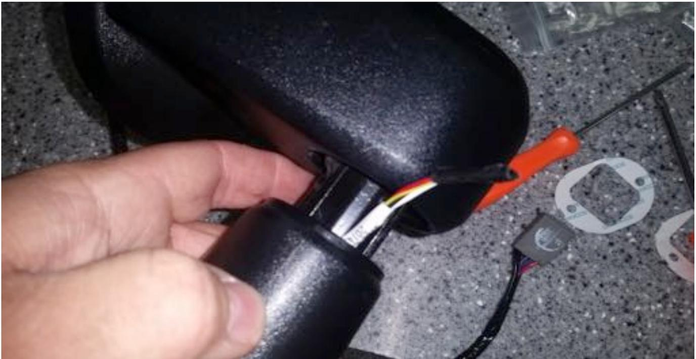
17. Following the factory harness run the camera harness through the mounting base and pull the rest of the camera harness through.
