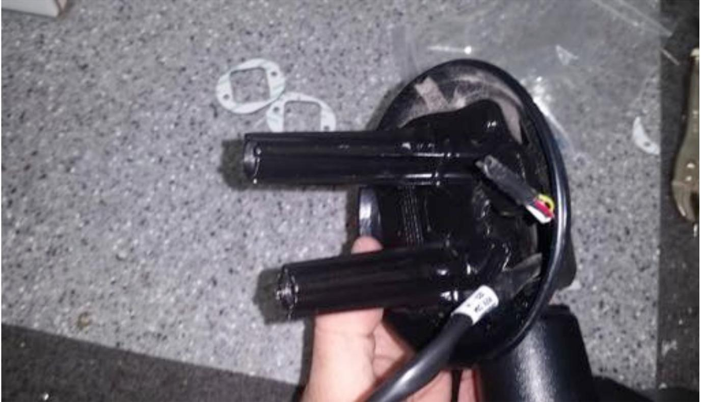
18. Attach the camera harness and the factory mirror harness to the pull wire that was already run through the door and pull the harnesses to the inside of the vehicle.
