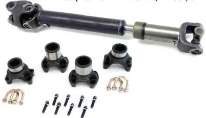
NOTES: Make sure that you align the balancing marks on the yoke and drive shaft at both the axle and the transfercase.
