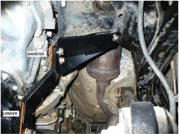
16. Use the supplied 3/8 bolts with a lock washer then a flat washer. Leave these bolts loose until all the other pieces are installed.
