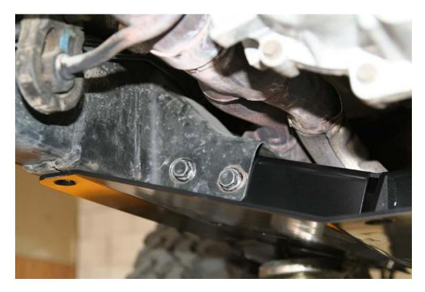
7. At this time, mark and drill the holes for the countersunk bolts. There are 4 total for the transmission skid.
