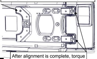
Open hinge, apply thread locking compound, torque bolts to 26 N-m (19 ft-lbs)
