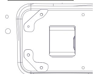
Note location of spacers, place gasket between spacer and tailgate. Apply thread locking compound and install bolts
