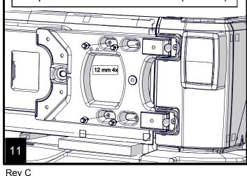
If installing the optional tire mount #77072345 in conjunction with cast hinge reinforcement kit, refer to instruction set K6862213 included with that kit. If reusing the factory tire mount, continue with step 14 in this instruction set.
