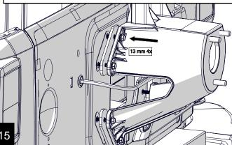
Torque 8 tire mount bolts to 20 N-m (15 ft-lbs) Remove support spacer under tailgate
