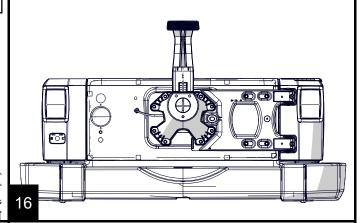
Optional: Push in the 7 rubber plugs into the threaded holes as shown.
