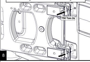
Install bolt to align cast hinge to tailgate. Visually inspect all bolt holes for alignment
