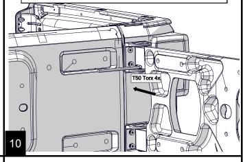
Apply thread locking compound, install and torque included bolts to 20 N-m (15 ft-lbs)
