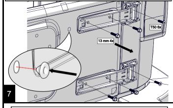
Apply thread locking compound, loosely seat original bolts into the hinges
