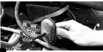
Run the cable as direct as possible to the throttle linkage from the firewall through the hollow screw you had assembled onto the "L" shaped bracket earlier. Install the cable housing onto the cable and into the head of the hollow screw. Note: You may need 2-3 5/16 flat washers so you can tighten down the nut shown in the picture below. Leave any excess cable to be trimmed at the end.
