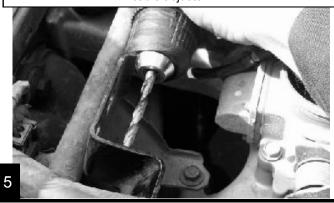
Mount the "L" Bracket and cable adjuster in such a way that it will pull the throttle linkage in the same direction as your accelerator pedal does.
