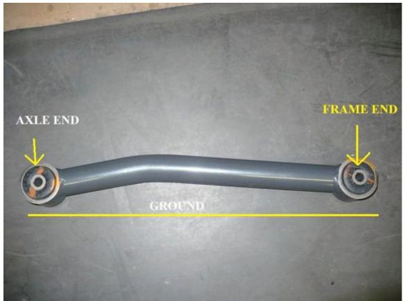
3. Tighten the factory control arm bolts to 125 ft-lbs. Be sure to torque bolts with vehicle's weight on the suspension as to not preload the control arm bushings.
