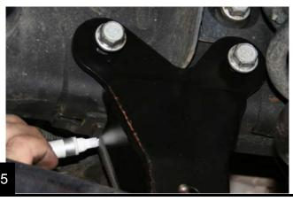
Place the new frame brace bar with the fixed end side into the factory trackbar location with the bend of the bar upwards. Insert a 9/16"x3.5" bolt into the top hole.
