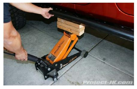
17. Using the factory hardware, secure your new LoD Signature Series Rock Slider to the points where the automatic transmisson and transfer case skid plates attach the frame rail on your Jeep JK Wrangler. An 18mm socket will be needed for this job.
