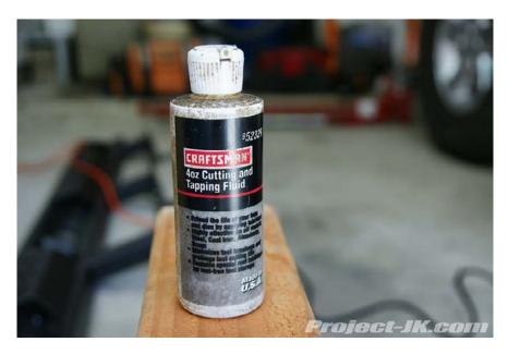
**15.** With the help of some cutting oil, slowly and carefully tap all your mounting holes. Due to the body of the Jeep JK Wrangler being in the way, you will not be able to use a standard tap handle to do this. I improvised and used a wrench to do this job.
