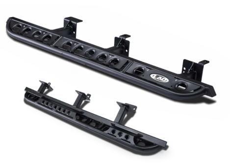
**1.** To remove either the Jeep JK Wrangler Unlimited Rubicon rocker guards or Sahara running boards, use a 10mm wrench to remove the 3 pairs of nuts securing them to the body pinch seam.
