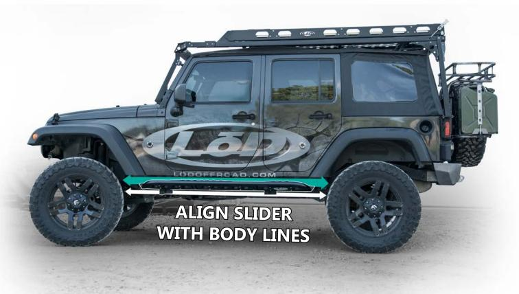
**Important:** Before marking or drilling any holes be sure to make sure that the slider is positioned properly. The slider needs to be aligned so that it maintains an even spacing between it and the pinch seam of the body.
