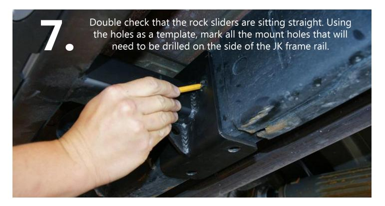
On the mount closest to the rear tire, there are two holes that will need to be marked off on the bottom as well.
