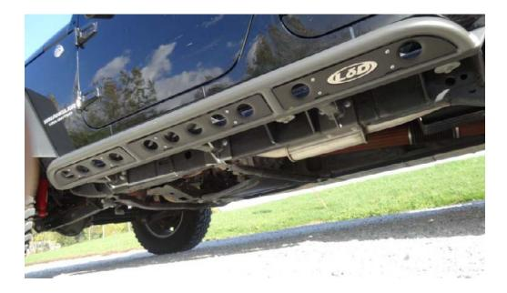
**20.** With both sliders installed on the Jeep install the lower side panels. Use the  $\frac{1}{4}$ " x  $\frac{5}{8}$ " button head bolts provided. The logo should be place to the rear of each slider as shown in the picture to the right.
