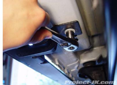
**3.** With the 6 nuts and 3 bolts removed, the factory rocker guards or running boards on your Jeep JK Wrangler Unlimited Rubicon or Sahara should pull off the body pinch seam with ease. Set them aside.
