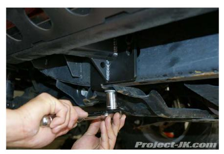
**18.** Using the 7/16"x1" bolts that come with the kit, secure your LoD Signature Series Rock Slider onto the new mouting holes that you made on your Jeep JK Wrangler's frame rails
