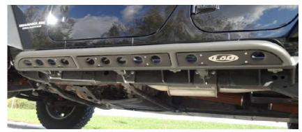
6. Using the factory hardware, secure your new LoD Signature Series Rock Slider to the points where the automatic transmisson and transfer case skid plates attach the frame rail on your Jeep JK Wrangler. An 18mm socket will be needed for this job. (Note: If your jeep has a manual transmission you will need spacers to make up thickness of this cross-member. If no spacers are used the sliders will not follow the body line.)
