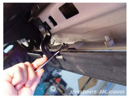
**2.** Using a 13mm socket, remove the 3 bolts securing the Rubicon factory rocker guards or Sahara running boards to the bottom of your Jeep JK Wrangler Unlimited's body.
