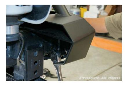
USING A 3/4" SOCKET, TIGHTEN UP THE LOD SIGNATURE SERIES WINCH PLATE FRAME RAIL MOUNTS AS SHOWN IN THIS PICTURE.
