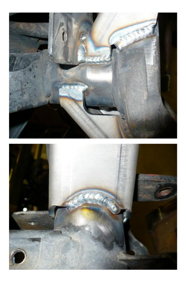
9. After welding, clean off any weld burrs and paint the desired color to prevent corrosion.
