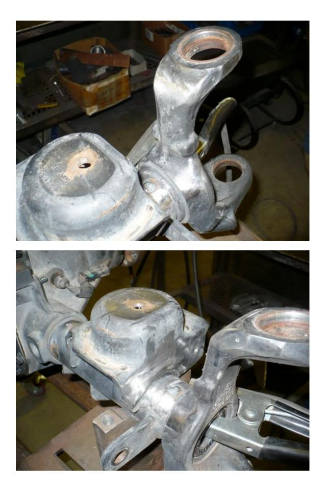
3. Once weld surfaces are prepared, place upper C-gussets in position. There will likely be a slight gap around the ball-joint area; use a C-clamp to tighten the gusset in the proper welding position.
