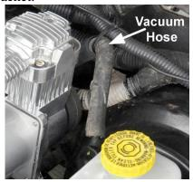
3. Loosely zip tie the vacuum hose as indicated in the previous picture, in order to assure at least ½" clearance around the compressor head.
