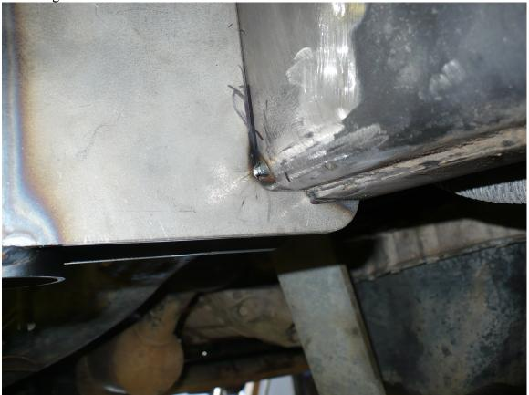
3. If you are not using air bumps and purchased the budget bump kit, cut the bump stop cup from the stock upper coil mount. Be careful to just cut the weld and leave the bottom of the cup intact. You will need a 3/8 x 1 coarse thread bolt and washer to attach the cup to budget bump.
