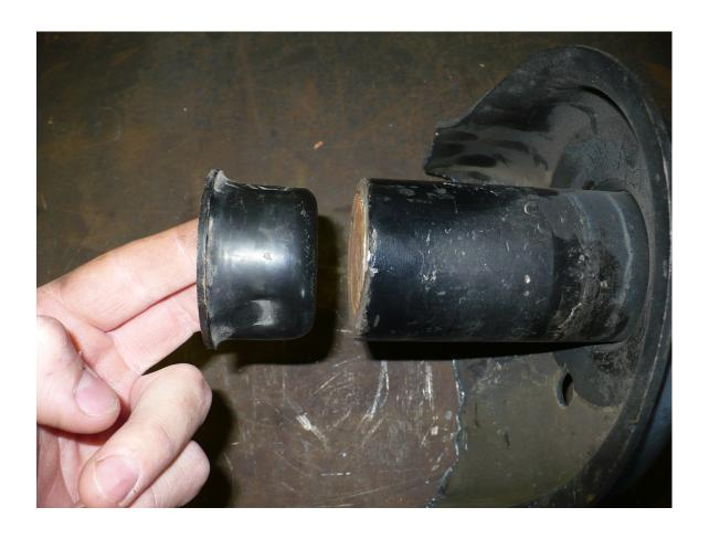
Install the snap ring in the lowest groove; this will give you the same collapsed length as an air bump.
