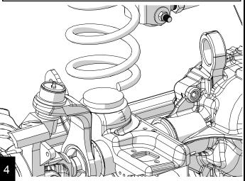
Using the center divot in the spring pad as a guid, drill a 5/16" hole. If necessary, remove the upper bumpstop to access the 15mm bumpstop bell retainer bolt. This will help gain drill access.
