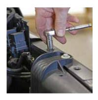
5. Loosen the Master Cylinder nut closest to the passenger side, using a 13mm socket and short extension. DO NOT REMOVE!
