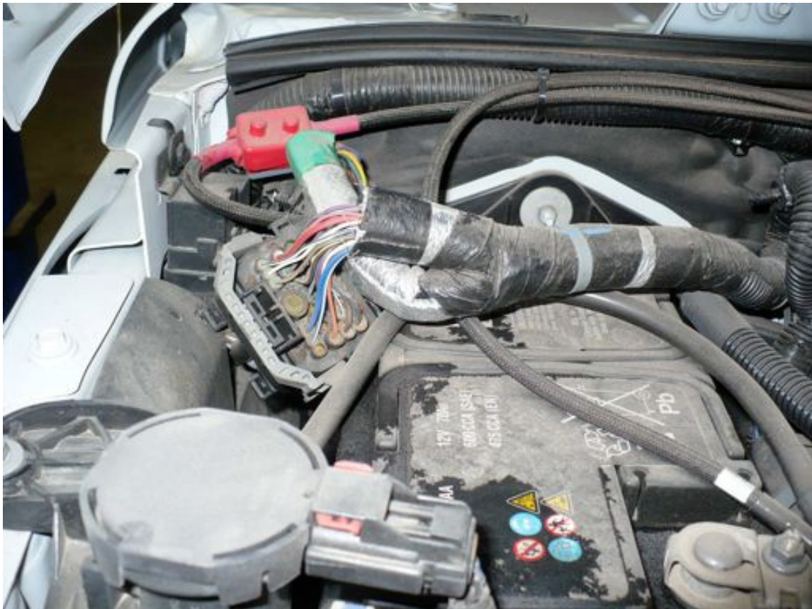
Pic 5.1; Factory wiring harness on a 2012 3.6L JK relocated from under the battery to above it.
