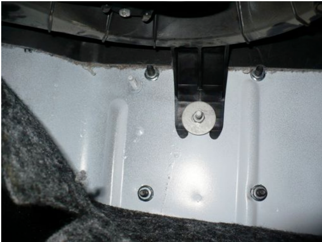
Picture 8.1; Backside of heat exchanger mounting on 2012 Jeep JK underneath the passenger foot well carpeting.
