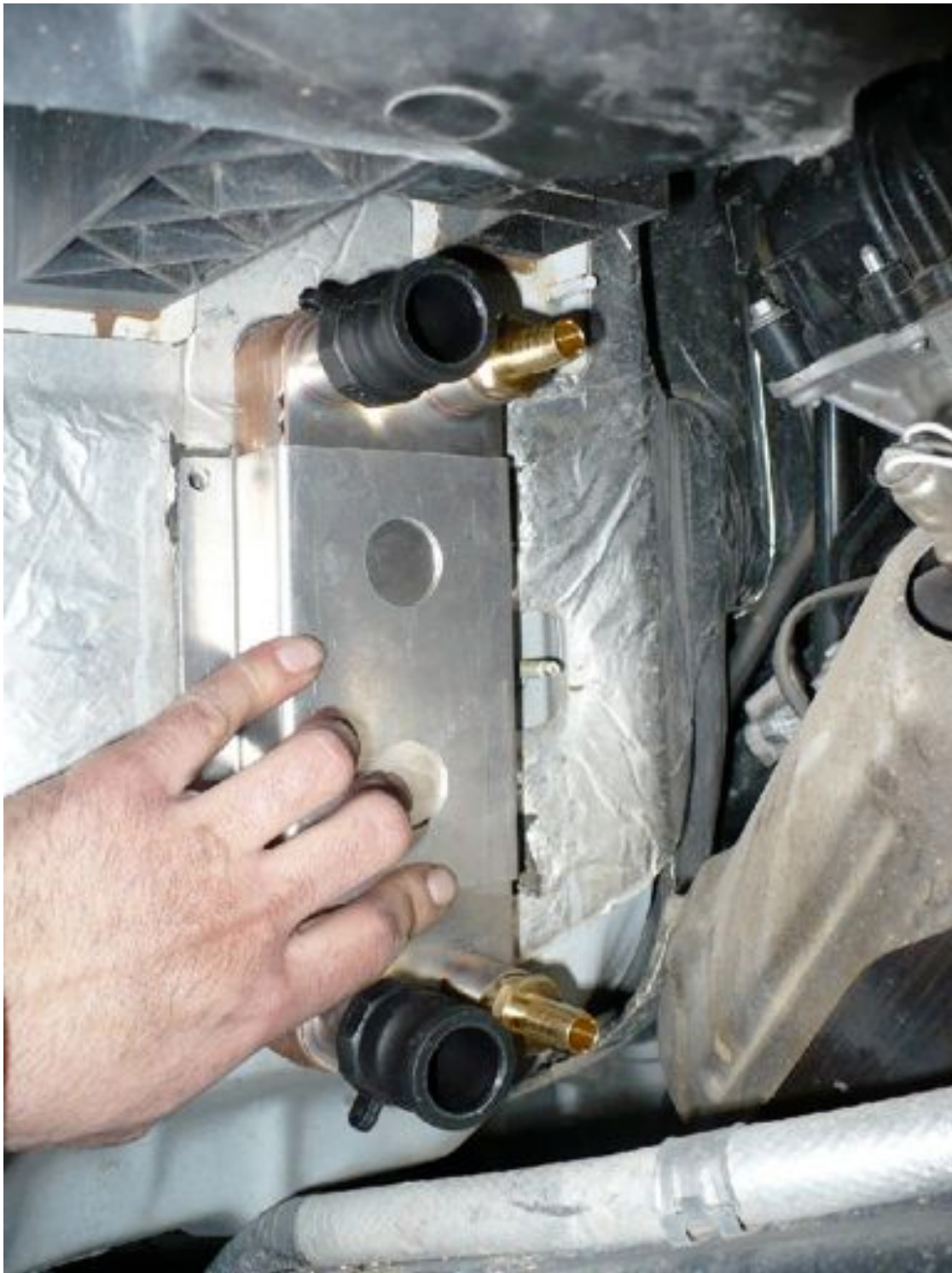
Picture 5.2; Heat exchanger assembly positioned on the passenger side firewall / inner fender well area.
