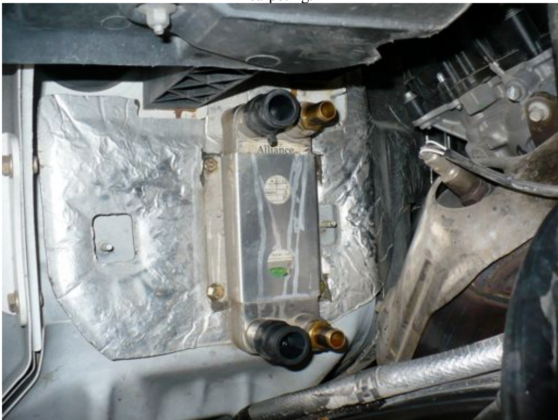
Picture 8.1; Backside of heat exchanger mounting on 2012 Jeep JK underneath the passenger foot well carpeting.
