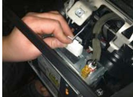
6. Remove (if plugged in) the 4-pin to 6-pin adaptor. It is not need for installation.
