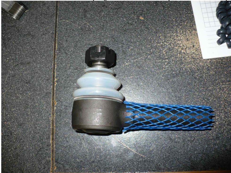
10. Tighten the castle nut by hand. You should be able to get three full revolutions of the nut without putting a wrench on it. If not, remove the flip adapter and enlarge the hole in the knuckle. Once the castle nuts are hand tightened, torque to 55 ft-lbs or more to align the cotter pin hole. Install the cotter pin on the steering arm end and bend the ends over. Do not install the cotter pin at the pitman arm side at this time.
