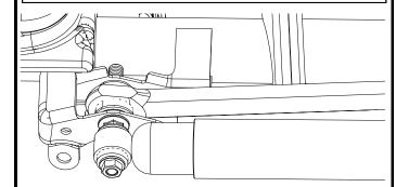
Make sure the tires are straight, then manually collapse the steering stabilizer to its centered position. Hint, use a tape measure. Make a mark on the tie rod where the stabilizer eyelet aligns with the tie rod. Note, if you are not relocating your stabilizer, it will be on the bottom of the tie rod.
