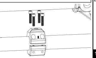
Use a 3/4" to install the remaining end of the stabilizer onto the top of the clamp using the 1/2" bolt and two 1/2" washers. Use Blue Loctite and Torque to 47ft-lbs.
