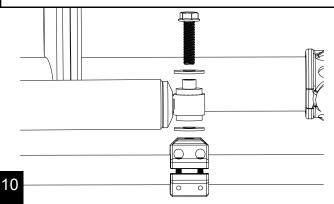
If you are not relocating your steering stabilizer, skip this step. Use an 18mm to tighten the sleeve nut.
