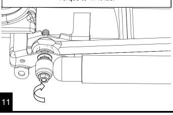
Have a second person SLOWLY turn the steering wheel lock to lock while you watch the stabilizer. Verify that the stabilizer clears all the components. Once clearance and position of the clamp have been verified, use a 3/16" allen wrench and tighten the 4 clamp bolts in a cross pattern to 6 ft-lbs.
