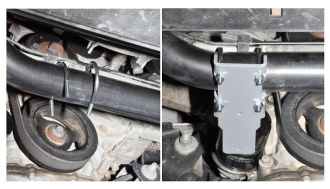
2. Place the tank mount bracket into position and firmly hand tighten all four nuts on the passenger side.
