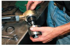
7. Completely remove the urethane bushing and ball from the joint.
