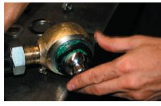
10. Place the large tool on the opposite side of the bushings pushing the bolt through to secure everything. Place the second half of the urethane bushing making sure to match up the notches.
