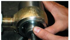
4. Place the provided washer and nut onto the threaded end of the bolt and begin tightening it until there is a little groove. Tighten just enough to release pressure in order to remove the snap ring.
