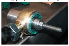
13. Pull the spiral snap ring slightly apart and begin laying it into place bottom first and wind it around so that the entire snap ring is in the groove.
