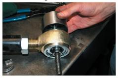
3. Slide the smaller of the two tools onto the threaded end of the bolt with the lip towards the joint so it will slide in tight against the washer inside the joint.
