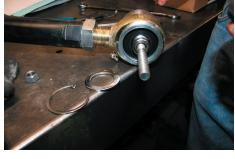
6. Now, to push out the urethane bushing, switch the larger of the tools to the side you just removed the snap ring and washer from. Switch the bolt and the small tool as well as the provided washer and nut to the opposite side and begin tightening to push the urethane out of the joint.
