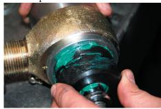
11. Place small tool, washer and nut on the threaded end of the bolt. Begin tightening the bolt to push the urethane back into the joint.
