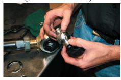
8. Place the washer back inside the joint before placing the new ure-thane and ball back into the joint. **Note:** As you begin replacing the bushing, it is important to grease each part as you insert it into the joint.
