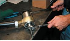
5. Remove the internal snap ring using snap ring pliers and then remove the internal washer as well.
