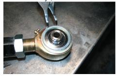
2. Put the larger of the two tubes on the side you just removed the snap ring from. Slide the long bolt through with the head on the same end as the large tool.
