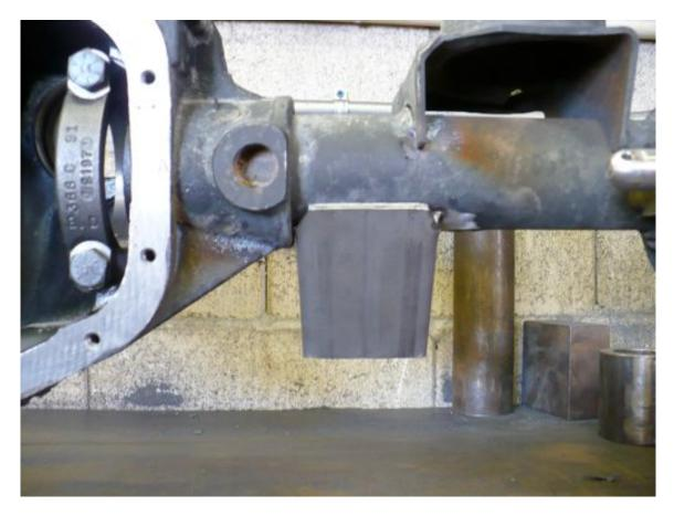
5. The bottom edge should be level or back edge vertical when the pinion is level or diff cover surface is vertical. Tack weld in place.
