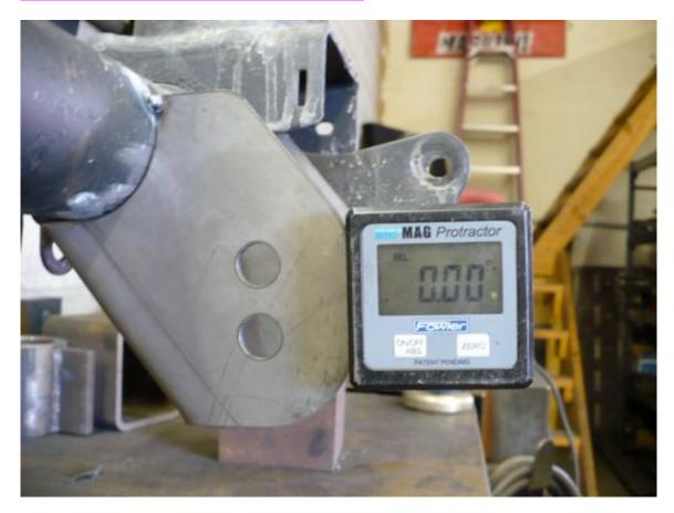
6. Position the passenger side bracket opposite. The easiest way is to measure from the machined edge adjacent to the weld on the inner C. Measure the driver side then make the passenger side bracket the same dimension. The dimension should be close to 5 ¼ to the outside edge of the new lower control arm bracket. Tack weld into place.
