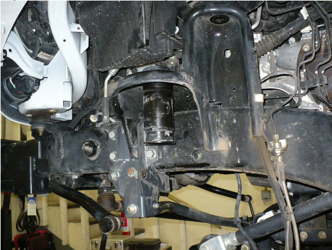
IMG 4.1 Front suspension tear down.
