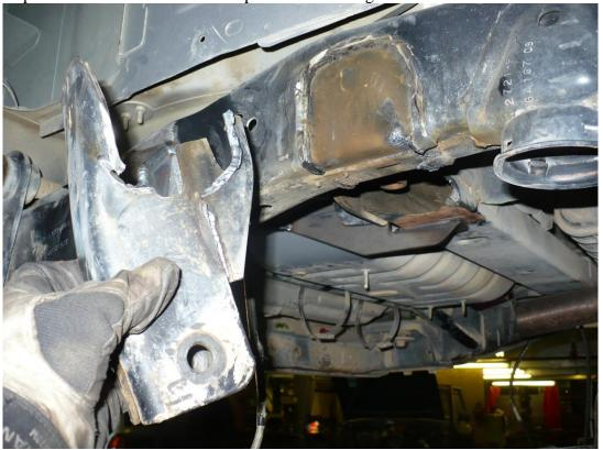
11) Now is the time to fully weld on all the new bracketry. Weld the 8032 RLCA Stretch Brackets wherever they meet the frame. See weld pictures below for reference.
