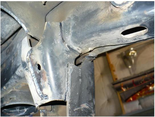
10) With the welds cut, remove the bracketkt. It should come off in more or less one piece as shown below. Clean up the area with a grinder.
