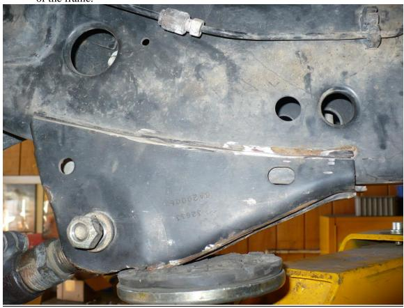
d) Cut off the upper control arm bracket as shown below
