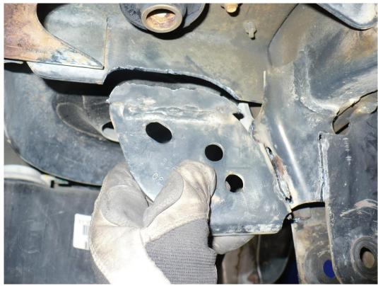
9) Next, using a 4-1/2" angle grinder with cut off wheel, cut on the weld of the remaining bracket. Be careful not to cut too far and cut into the frame.
