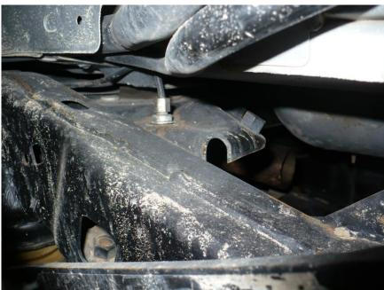
b. Factory JK rear bump stops can be retained. Simply cut them off the frame at the weld and relocate 8" back. Pictures below show factory bump stop and 2" BS spacer.
