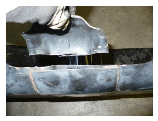
3) With stock control arm brackets removed, fitment of the 8032 RLCA Stretch Brackets can begin. These brackets are self locating via the body mounts. Fit them to the chassis as shown below. Snug bolts and clamp bracket to frame as shown.
