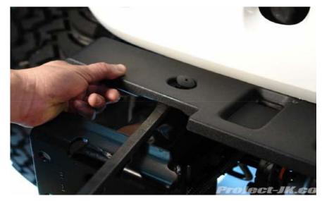
AGAIN, IF YOUR JEEP CAME EQUIPPED WITH FACTORY FOG LIGHTS, USE A PHILIPS SCEWDRIVER TO REMOVE THE 4 SCREWS SECURING THEM TO THE BUMPER. THEN, PULL THE FOGLIGHTS OUT AND SET THEM ASIDE UNTIL YOU ARE READY TO INSTALL THEM IN YOUR NEW BUMPER.
