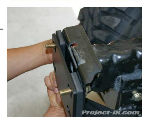
WITH THE HELP OF A FRIEND, CAREFULLY PLACE YOUR NEW LOD SIGNATURE SERIES SHORTY BUMPER ONTO THE FRAME RAILS OF YOUR JEEP AND SLIDE THE MOUNTING BOLTS THROUGH THE HOLES. REACHING FROM THE BACK, LOOSELY SECURE IT IN PLACE USING THE NUTS PROVIDED.
