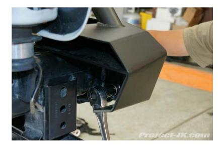
USING A 3/4" SOCKET, TIGHTEN UP THE LOD SIGNATURE SERIES WINCH PLATE FRAME RAIL MOUNTS AS SHOWN IN THIS PICTURE.
