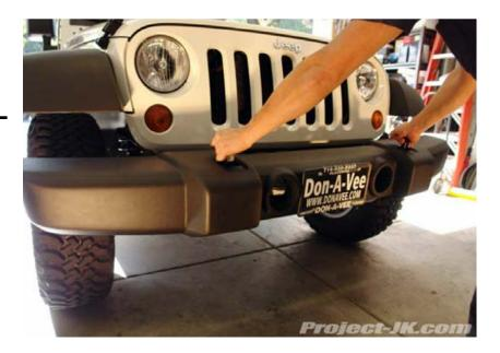
USING A PHILLIPS SCREWDRIVER, REMOVE THE TWO PLASTIC SCREWS SECURING THE TOP PLASTIC COVER IN PLACE.
