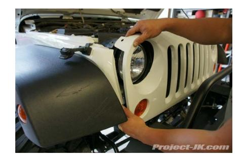
ONCE LOOSE, THE ENTIRE PLASTIC SCREW AND EXPANSION SLEEVE SHOULD PULL UP AND OUT OF THEIR MOUNTING HOLES.
