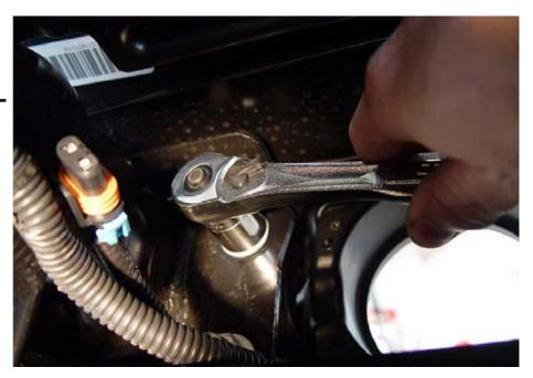
USING AN 18MM SOCKET, REMOVE THE 4 BUMPER MOUNTING NUTS (2 ON EACH SIDE) LOCATED NEXT TO THE OUTSIDE OF YOUR JEEP JK WRANGLER'S FRAME RAILS.
