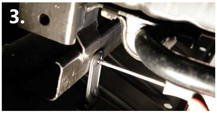
Now, climb under the front of your JK Jeep Wrangler and using a philips screwdriver, remove the two remaining plastic screws securing the air dam to the lower cross member. As before, if these screws spin, just use a flathead screwdriver to pry them out.
