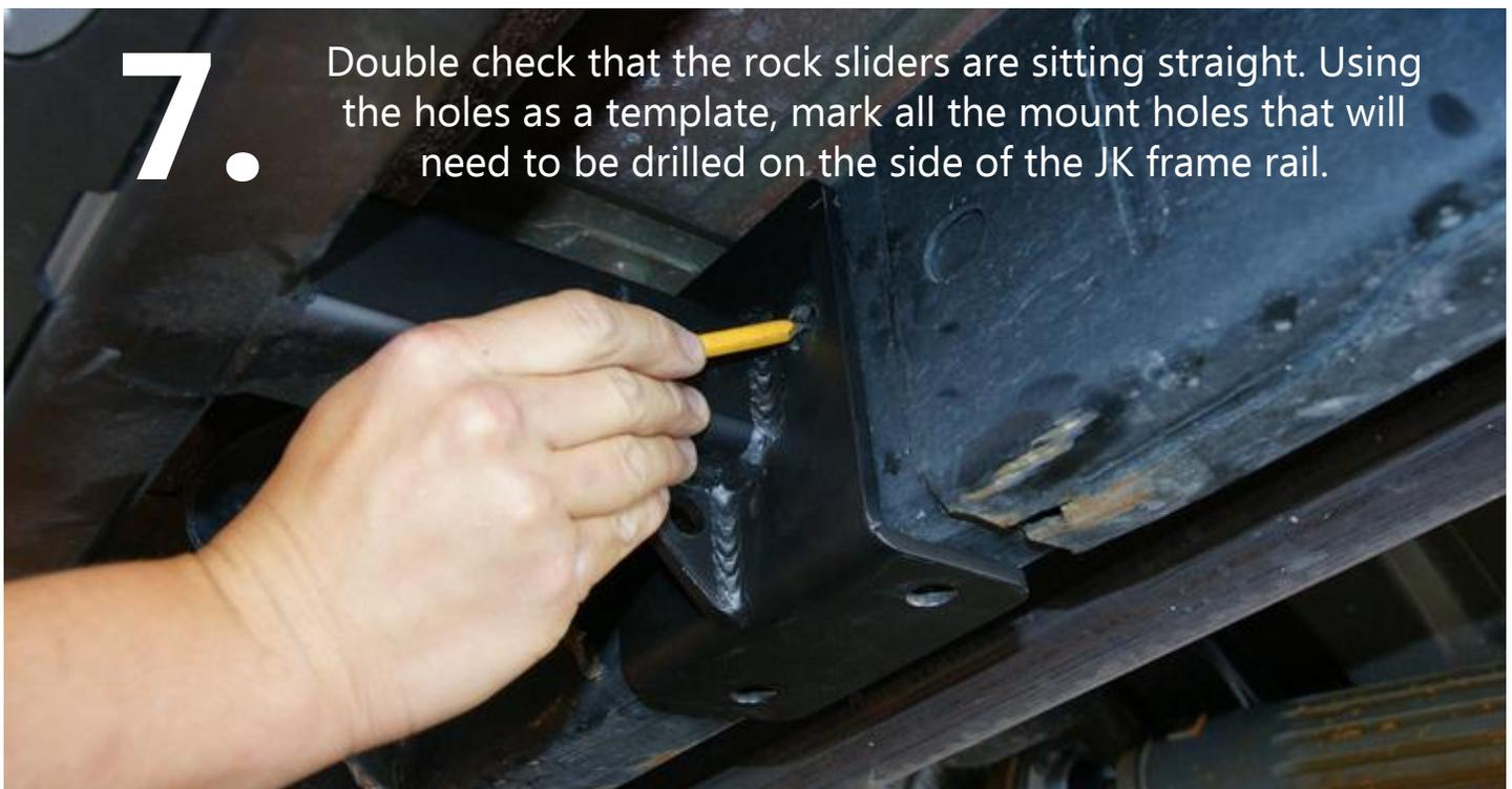
7. Double check that the rock sliders are sitting straight. Using the holes as a template, mark all the mount holes that will need to be drilled on the side of the JK frame rail.
