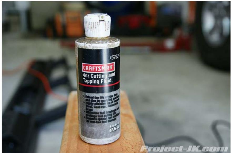
**15.** With the help of some cutting oil, slowly and carefully tap all your mounting holes. Due to the body of the Jeep JK Wrangler being in the way, you will not be able to use a standard tap handle to do this. I improvised and used a wrench to do this job.
