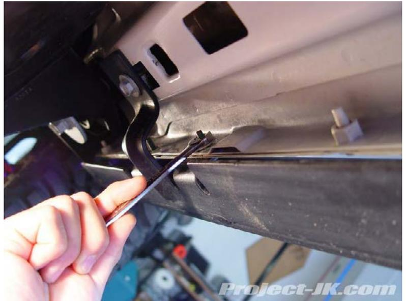
**2.** Using a 13mm socket, remove the 3 bolts securing the Rubicon factory rocker guards or Sahara running boards to the bottom of your Jeep JK Wrangler Unlimited's body.
