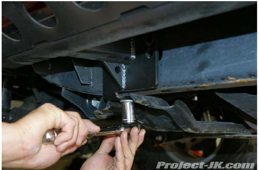
**18.** Using the 7/16"x1" bolts that come with the kit, secure your LoD Signature Series Rock Slider onto the new mounting holes that you made on your Jeep JK Wrangler's frame rails
