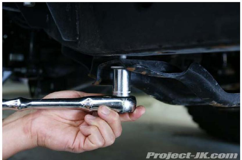
**5.** Maneuver your LoD rock sliders into place underneath the jeep. The rear mount of the sliders has 4 bolt holes so the sliders will need oriented so that the mounts with 4 holes are to the back of the Jeep.
