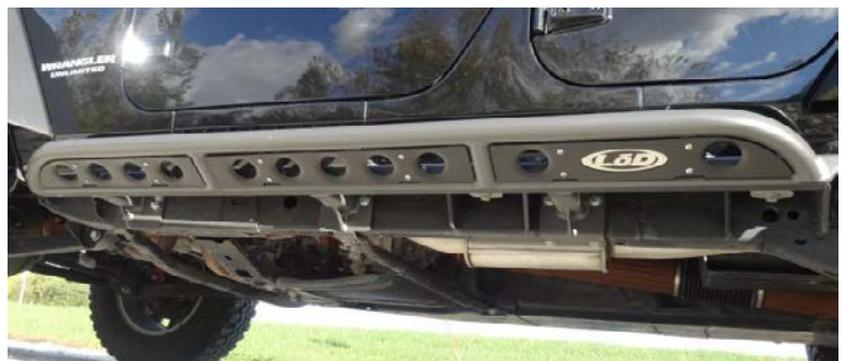
6. Using the factory hardware, secure your new LoD Signature Series Rock Slider to the points where the automatic transmission and transfer case skid plates attach the frame rail on your Jeep JK Wrangler. An 18mm socket will be needed for this job.
