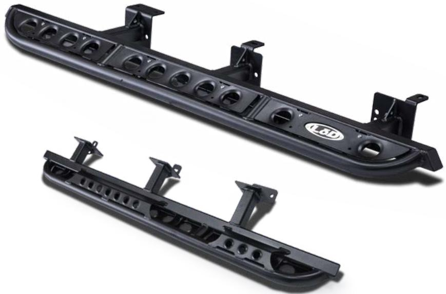
**1.** To remove either the Jeep JK Wrangler Unlimited Rubicon rocker guards or Sahara running boards, use a 10mm wrench to remove the 3 pairs of nuts securing them to the body pinch seam.
