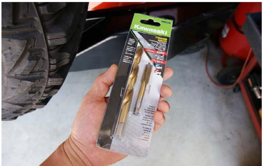
**13.** Using the drill bit that comes with the drill and tap set, finish drilling out all the pilot holes that you made back on step #11.
