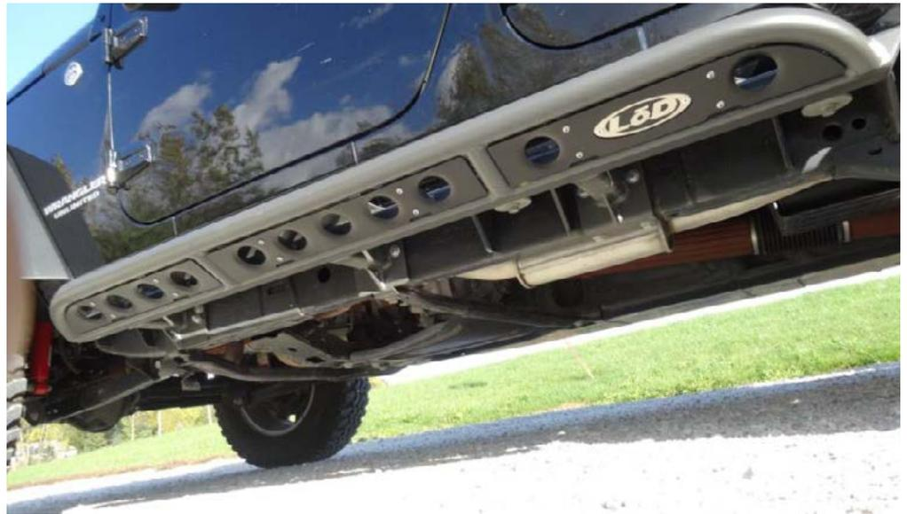
**20.** With both sliders installed on the Jeep install the lower side panels. Use the 1/4" x 5/8" button head bolts provided. The logo should be placed to the rear of each slider as shown in the picture to the right.
