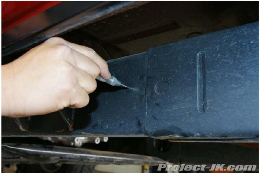
**11.** Using a small metal drilling bit or Unibit, begin drilling pilot holes on all the mounting points on you've marked off your Jeep JK Wrangler's frame rail.
