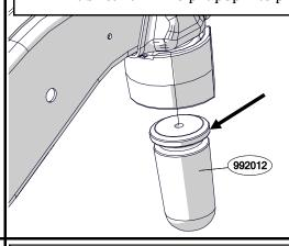
Locate the rear lower bumpstop pad (954600) and position pad with the extended end facing the front of the Jeep, as shown.
