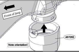
On Jeeps with slightly larger bumpstop bell housings the cup will be a tight fit. To help with this use a hand file and smooth any sharp edges on the bumpstop bell. Also apply a thin layer of grease to the cups inside lip. Then with a mallet give the cup a few quick taps to aid in installation.
