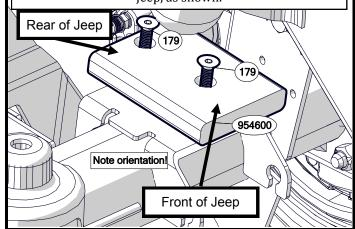
Each pad will receive two 179 bolts and two 630 Nylock nuts. Finish up the installation by torqueing each of the 4 fasteners to 7 ft-lbs (9.5 Nm).
