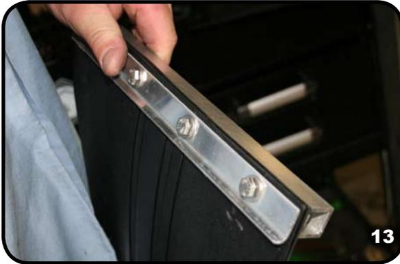
12. Place the mud flap on the mounting bar and install the locking nuts on the back of the bar. Make sure that you do a left and right mud flap. (Photo #14)
