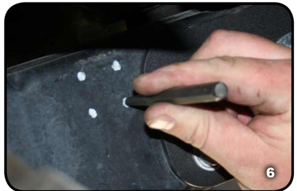
6. Drill out four holes with a 17/64 drill bit.(Photo #7,8)
