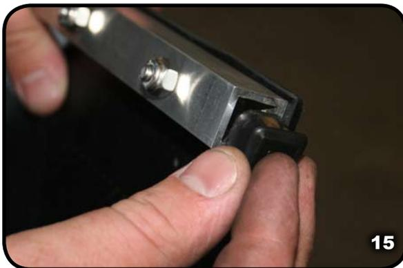
14. Place bar into mounting bracket and hold it up to the frame and see where it looks good. Remember these are universal mud flaps so
