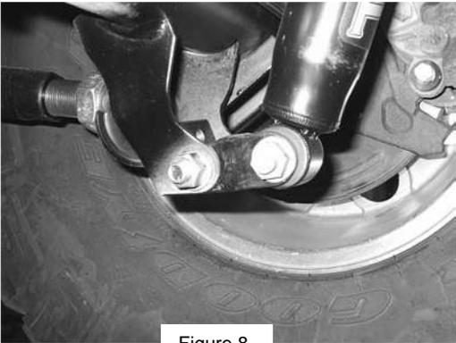
Install the extended brake line hose and the extended sway bar links. Mount
