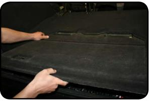
2. Remove the tail gate seal by removing the left side trim retainers with a removal tool and pulling the seal off of the body. (Remove the factory sub if equipped)
