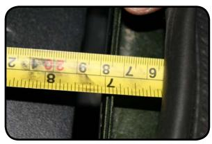
5. The top right side of the bracket should be 1-3/4" from the first rib in the floor. Measure from the radius at the top of the rib.
