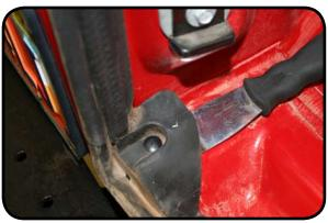
3. Lift the carpet up in the rear and support it with bungee cords or equivalent to reveal the floor.
