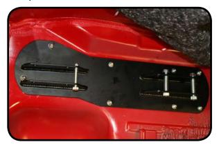
14. After the brackets are bolted down, lay your side carpets back down and cut out the carpet where the new seat tabs are. Then lay the floor piece down and trim the carpet where the tabs hit the carpet. The best way to cut out the carpet is to feel with your finger where the top of the tab is and cut along it with a sharp knife.
