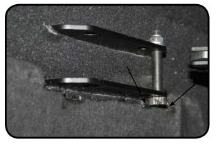
17. Once the lid clears the bolt you can install the front tab bolts into the front two big holes. Install the lock nuts and torque to 35 ft-lbs. Make sure that all of the bolts are nut side out.
