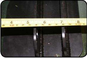
7. Mark the center of the holes and use a center punch to ensure accurate hole location.
