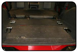
18. After all the bolts are torqued you can install the seat by placing the seat latch on the front two bolts and pulling down to latch the rear.
