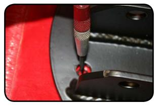
8. Place the right bracket in and locate it by measuring 7" from the outside pinch weld to the rear of the bracket once bracket depth is located measure from side to side it should be 34-1/4" from outside tab on left bracket to outside tab on the right bracket. (If you have a factory sub you need to cut the mounting stud flush with the floor)
