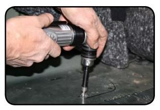
11. After the holes are drilled clean them out with brake clean or equivalent and silicone the nutserts and place them in the holes and use a nutsert install tool to lock the nutserts into place.
