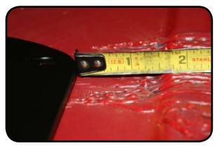
6. The rear of the bracket should be 5 -1/4" from the left wall of the body to the bolt tab.
