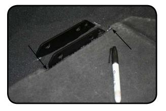
16. Install the small seat latch bolt into the rear tab in the front hole, with the nut towards the body side, and mark around the bolt head and trim out the lid for clearance.
