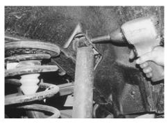
26. Disconnect the rear shocks. If you plan to replace the shock, you can remove the shock completely.
