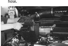
4. Pull the air filter assembly from the vehicle and set aside.
