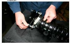
20. Lift the strut assembly into position. Attach the four top nuts using the new nuts and washers. Reassemble the fork to the bottom of the strut.
