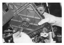
11. Disconnect the battery sensor from the bottom of the battery tray.
