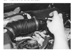
Loosen the hose clamps to remove the air box from the air intake hose.
