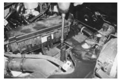
10. Be careful not to break any electrical wires that are attached to the battery tray. The connectors that attach the wires to the tray can be easily disconnected.
