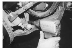
22. A jack stand is a convenient way to raise the knuckle into position so that the upper A-arm can be connected to the knuckle. Torque to factory specifications.
