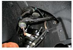
Note:If necessary remove lower A arm bolts to allow more droop.
