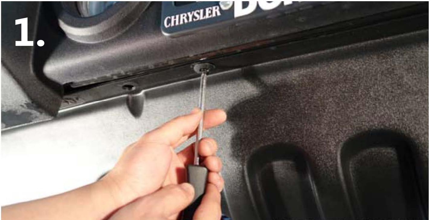
Begin the installation of your new LoD signature series shorty front bumper by unscrewing the 4 plastic screws securing the factory air dam to the bottom of your front bumper. a phillips screwdriver will be needed for this job.
