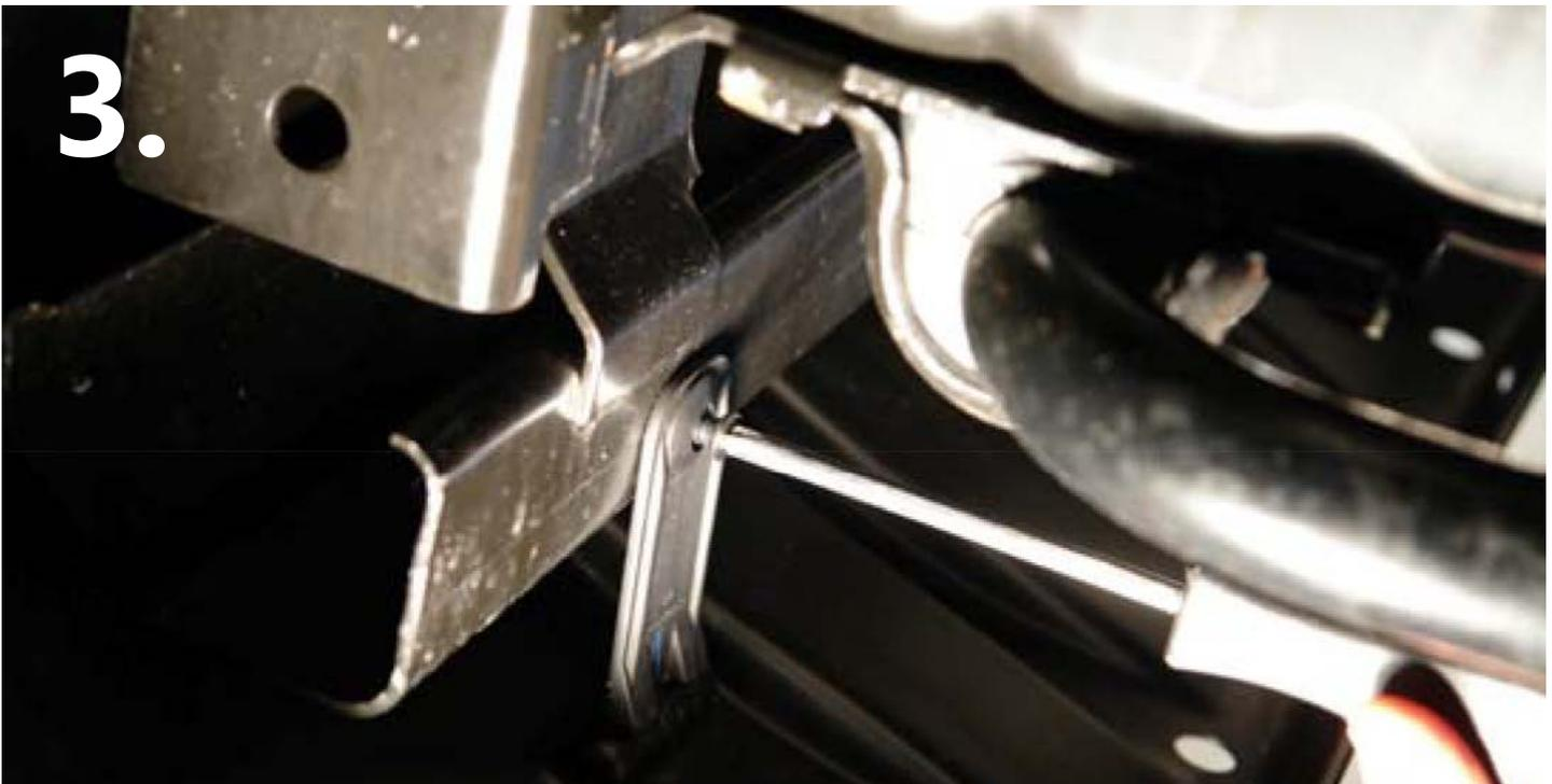
Now, climb under the front of your JK Jeep Wrangler and using a philips screwdriver, remove the two remaining plastic screws securing the air dam to the lower cross member. As before, if these screws spin, just use a flathead screwdriver to pry them out.
