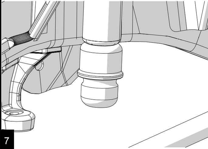
Install the spring and loose spacer as an assembly. Reinstall the new spacer retainer bolt.
