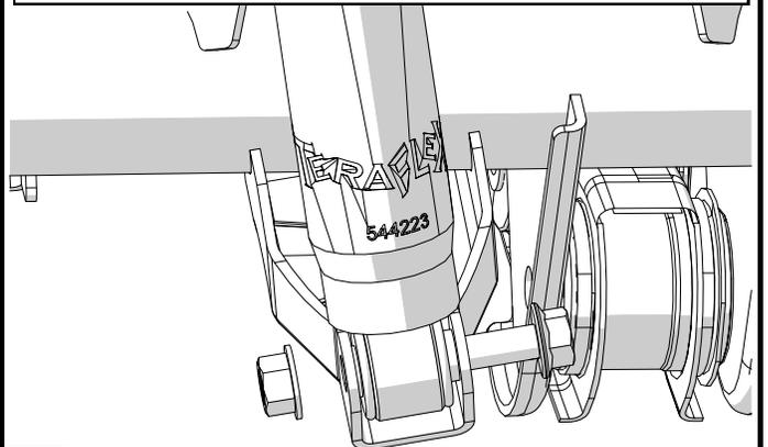
Remove the rear springs. (See Springs/ Rear Removal 999187)
