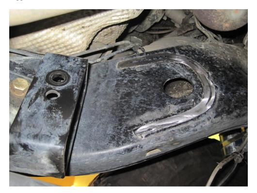
6) Remove the threaded inserts for the transmission skid plate. These are located on the bottom of the frame just to the rear of the stock lower control arm brackets. Thread the skid plate bolts into the threaded inserts so there is about a ½" of thread showing. Strike the head of the bolt upward with a large hammer to break the threaded insert loose from the frame. Remove the threaded insert and bolt.
