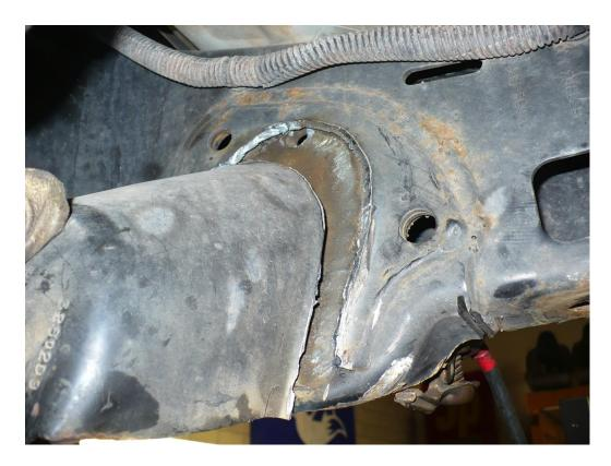
3) Using a cut-off wheel, cut the outer part of the lower control arm bracket as shown below. Be careful to not cut through the frame.
