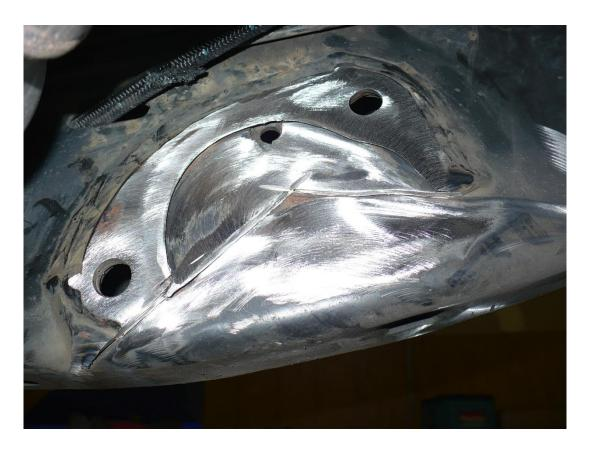
5) Cut off the upper control arm mount from the frame
