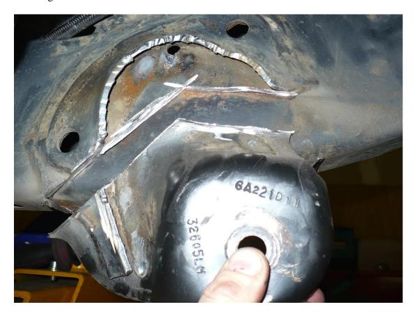
4) Grind the cut edge off of the remaining part of the lower control arm bracket on the inner frame. Do not remove this section of the factory lower control arm bracket. You need retain the two layers of brackets welded to the frame for the proper spacing of the new control arm brackets.
