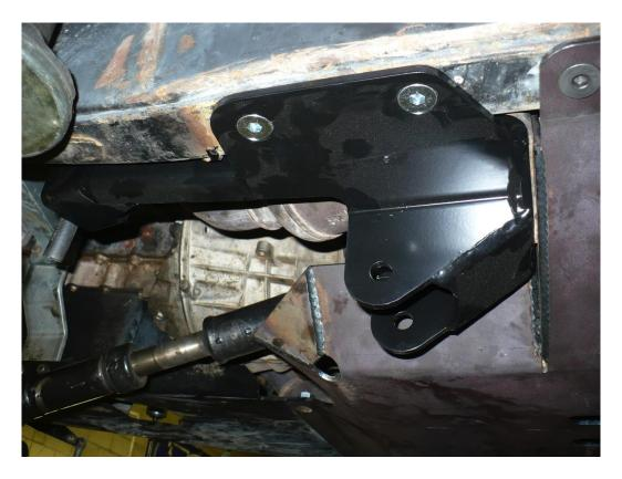
11) Install the nuts to the transmission cross member bolts, loosely tighten to bring the control arm bracket against the front of the transmission cross member.
