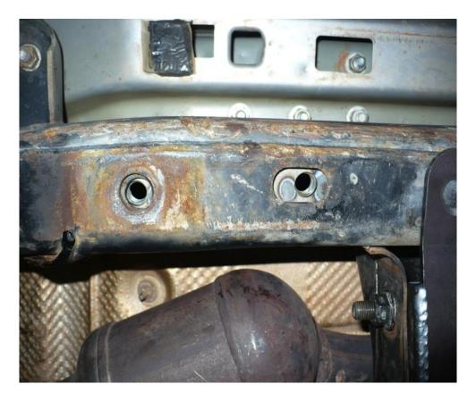
9) Remove the nuts from the transmission cross member bolts (1). Make sure the nuts are on the front side of the cross member, if not, flip the cross member bolts around.
