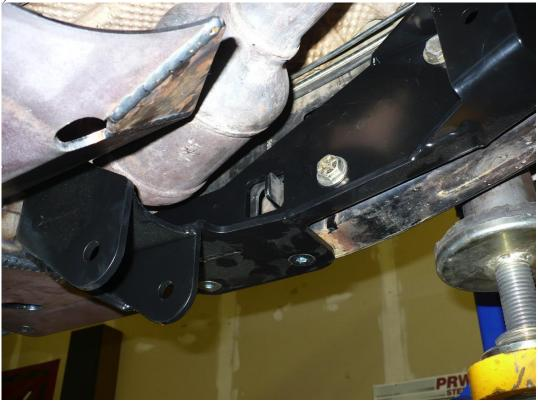
13) Tighten all the hardware for the control arm brackets to 90 ft-lbs <u>Installation is Complete</u>
