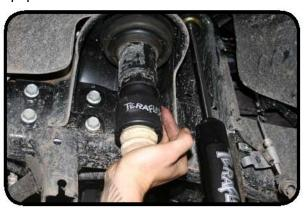
29. Install new 3 inch coil springs. Do the drivers side first.
