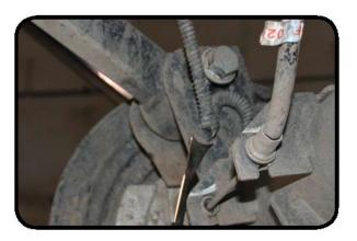
Disconnect the brake line bracket at the frame using a 10mm socket. DO NOT DISCONNECT THE BRAKE LINES FROM THE CALIPERS.
