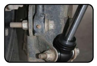
17. Install new rear bump stop spacer by placing the spacer on the axle pad. The extended part of the pad facing forward. Use the provided 5/16" x 1 1/4" bolts with 5/16" washers and 5/16 nuts. Tighten with 1/2" wrenches.
