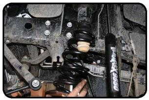
Install the new sway bar links, on the outside of the sway bar and inside of the axle mount. Torque to 75 ft-lbs.
