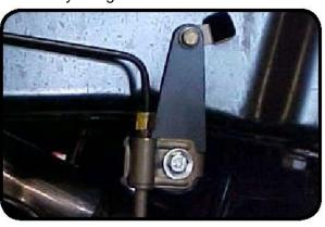
19. Install the new rear track bar bracket by removing the lower control arm bolt. Place the bracket into place, reinstall the control arm bolt. Install the supplied bolt and sleeve into the factory track bar location. Using the supplied u-bolt and nuts install the u-bolt around the axle tube. Torque the u-bolt nuts to 85 ft-lbs and the supplied bolt to 75 ft-lbs.
