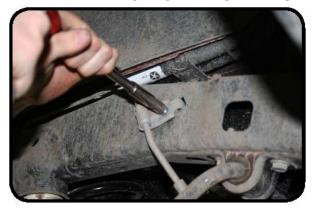
Remove the bracket that holds the park brake cables to the body using a 10mm deep well socket.
