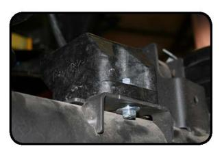
18. Install rear brake line extensions provided in the kit. Bolt the bracket to the factory brake line bracket by removing the 10mm bolt and installing the bracket in that location with the bend of the bracket going flush with the frame. NOT STICKING OUT AWAY FROM THE FRAME. Torque to 14 ft-lbs. (If bracket gets installed the wrong way it will rub on your tires) Then use the supplied hardware to attach the factory bracket to the drop bracket by using 1/2" socket and wrench.
