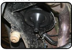
13. Install the factory isolator on the new spring guide spacer. Don't forget to reuse the factory spring isolator. If the isolator is left out your ride height will be about 1/2 inch lower in the rear. The isolator also helps dampen noise.
