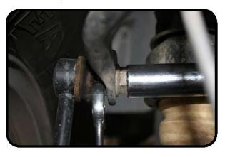
Remove the clips that secure the ABS wiring harness to the upper control arm mount.
