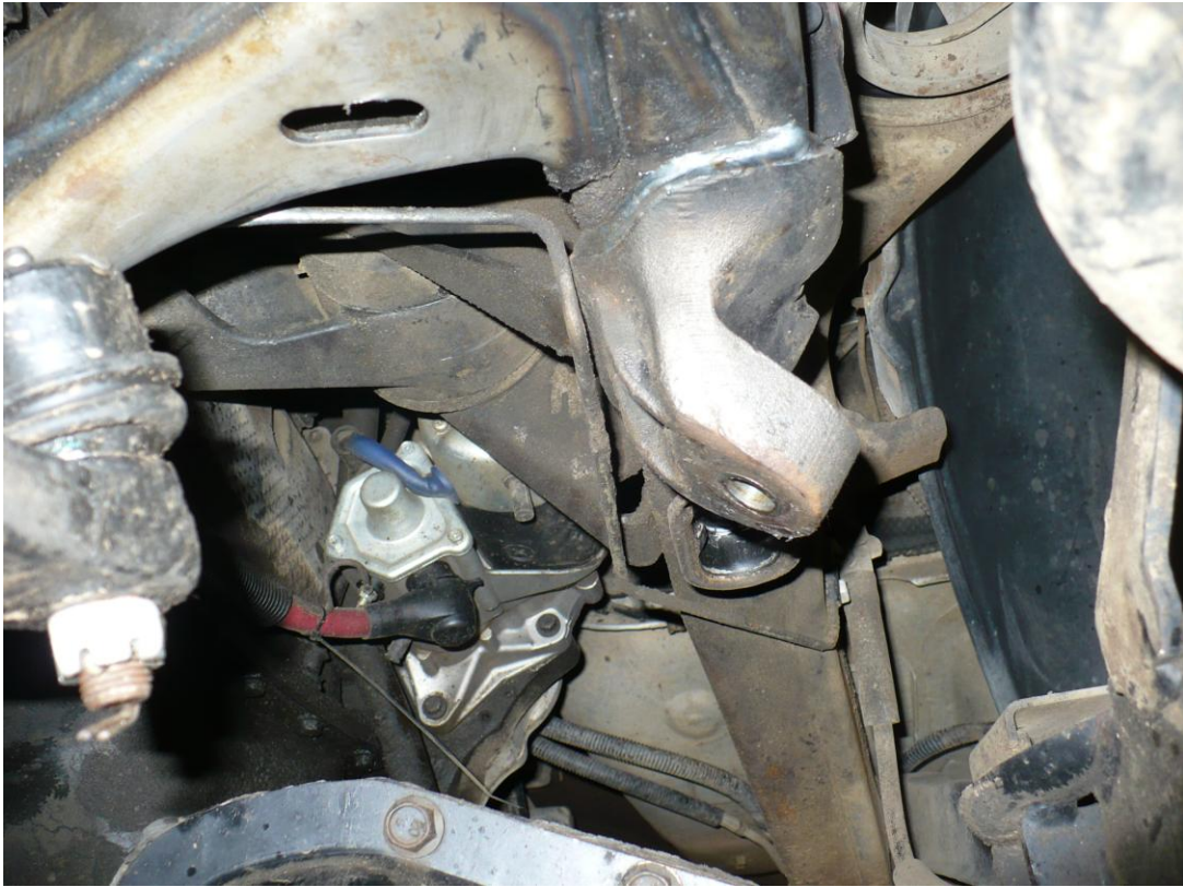
Picture 4.2 (TB bracket that will require no grinding modifications)
