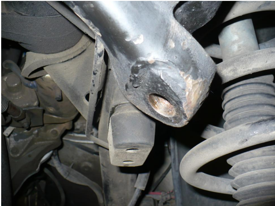
Picture 4.1a (Underside view of TB bracket that will require grinding)
