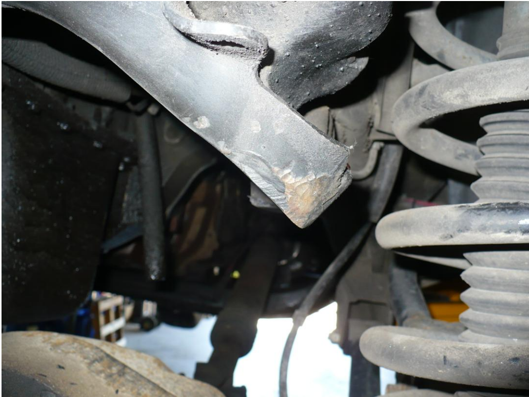
Picture 5.1b (Front view of factory TB tab, note smooth surface for conversion bracket to rest on.)
