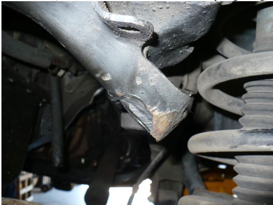
Picture 4.1b (Front view shows uneven surface that needs to be cleaned up)
