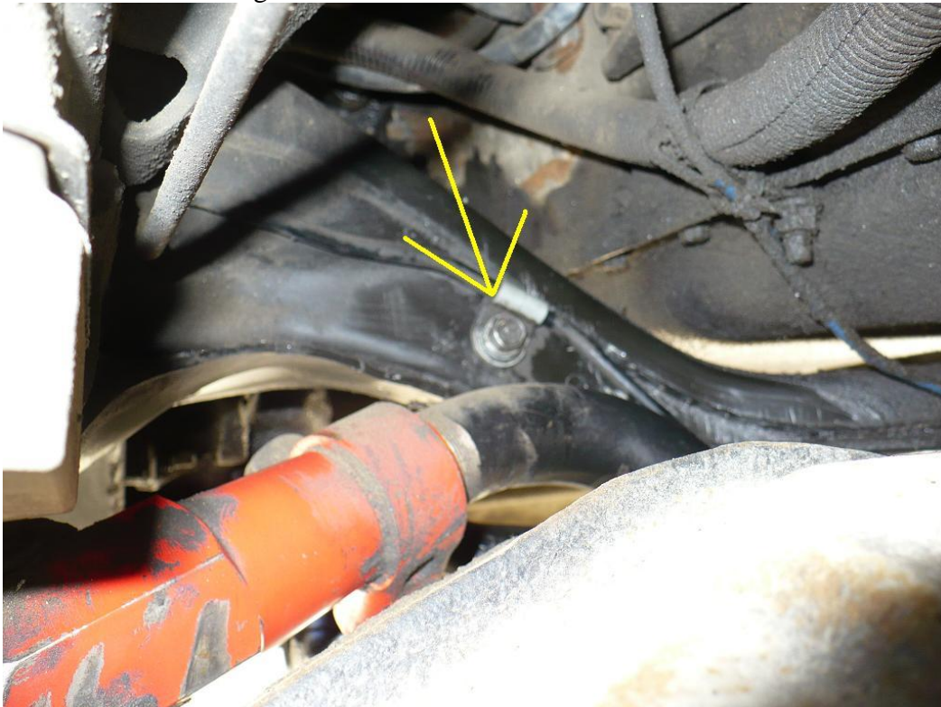
Picture 5.1b (Front view of factory TB tab, note smooth surface for conversion bracket to rest on.)
